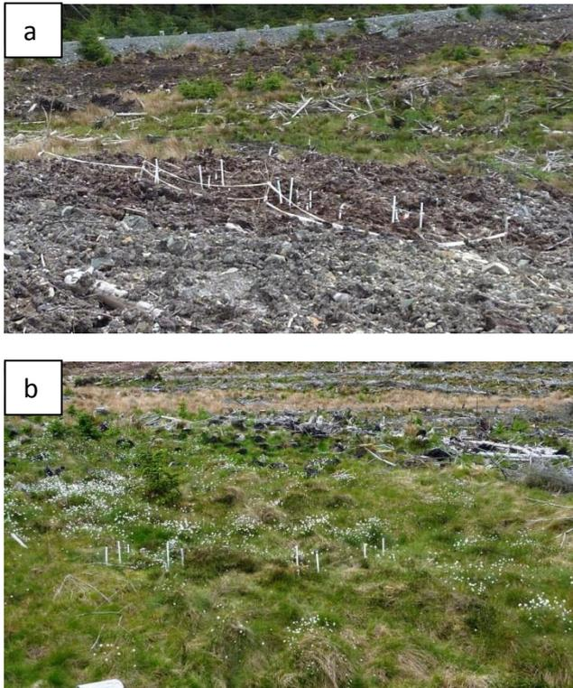
**Figure 92. a) Peat store and b) control site at Arecleoch wind farm. Nests of piezometers are visible distributed across the area.**
