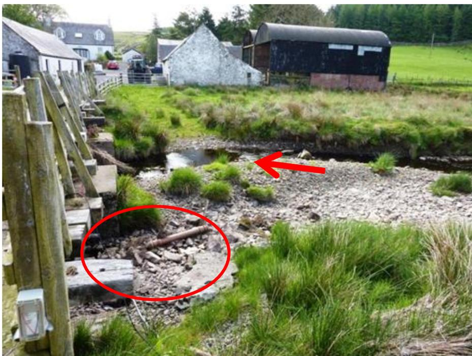
**Figure 33. Crosswater of Luce sample point during a prolonged dry period showing exposed instrumentation within the red circle. Water flowed only in a channel on the far side of the gravel bar (indicated by the arrow)**
