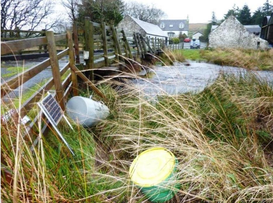
**Figure 34** Crosswater of Luce sample point during high flow conditions showing the automatic sampler dislodged and separated from its green and yellow stand.
