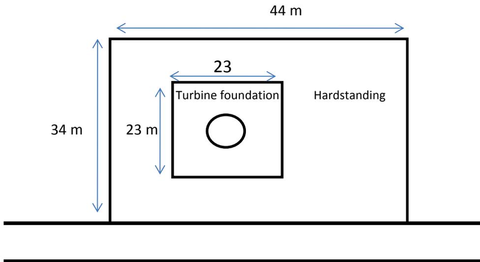
Figure 51. Schematic of the dimensions of a typical turbine base excavation
