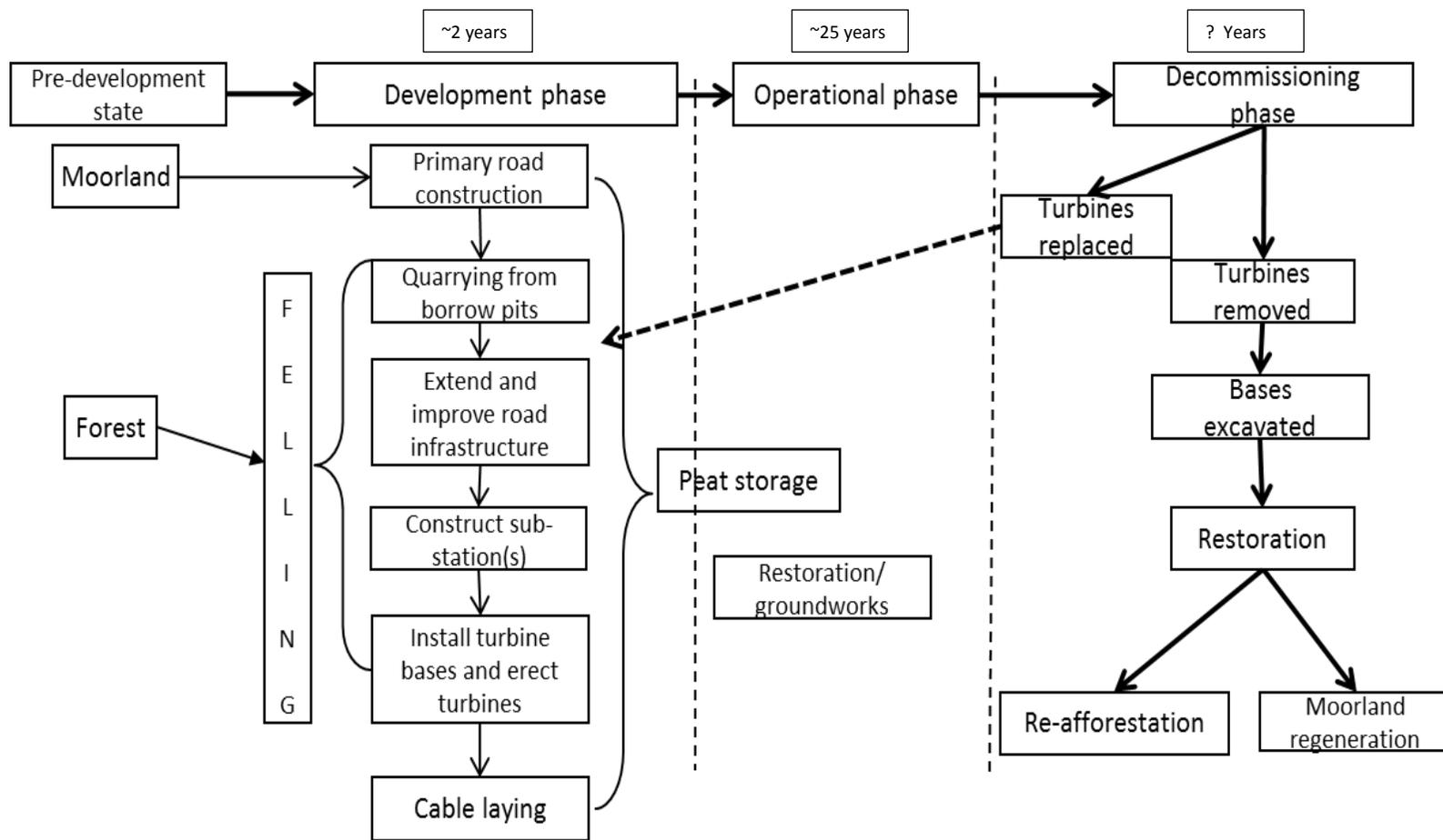
Figure 50. The wind farm cycle. The starting point is assumed to be either moorland or forest. In the case of the latter felling will extend across the development phase activities grouped in the {. Peat storage may take place as a result of excavations from all development phase activities and can extend into the operational phase if all the excavated peat is not reused.
