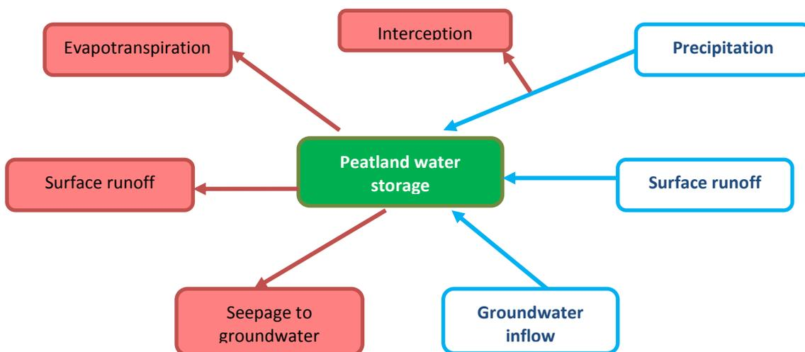
**Figure 20. A peatland water balance. Labels in red indicate processes by which water leaves a peatland. Labels in blue indicate processes that add water to a peatland (from Charman 2002).**
