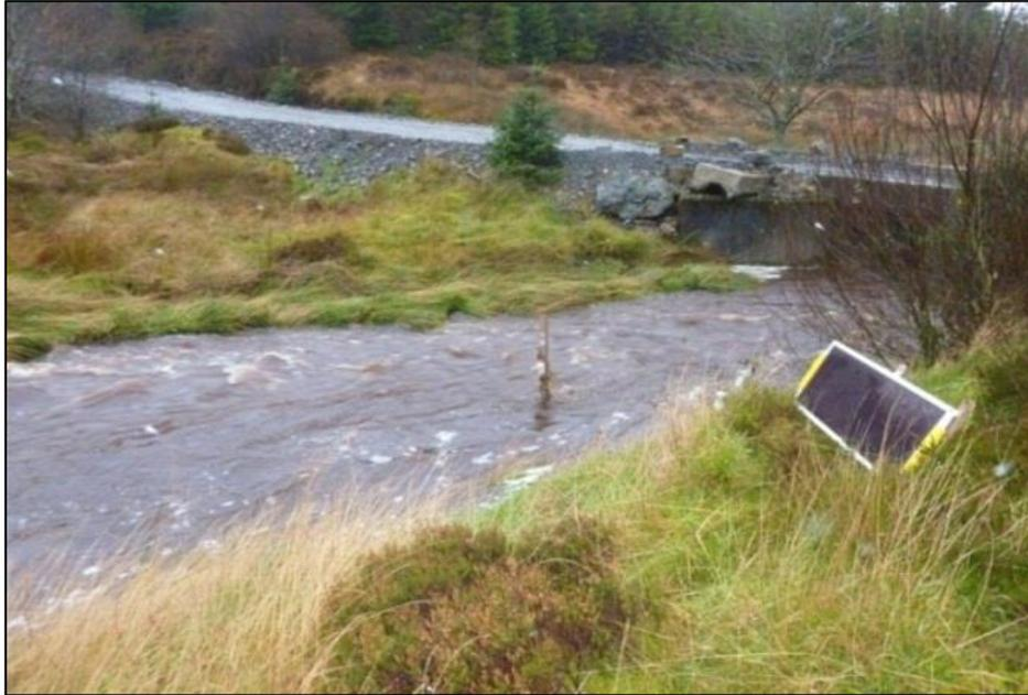
**Figure 19. Tig sample point – a cobble/boulder bed stream in the heart of Arecleoch forest. The solar panel used to trickle charge the autosampler battery is visible in the foreground**
