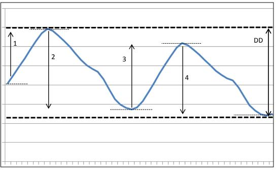
Figure 3.1: A comparison of how 'drawdown' (DD) and 'aggregated water level change' (Sum of 1-4) are calculated, on reservoir height, time graph
