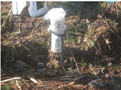
**Figure 4-3: NaI detector supported at ground level.**
