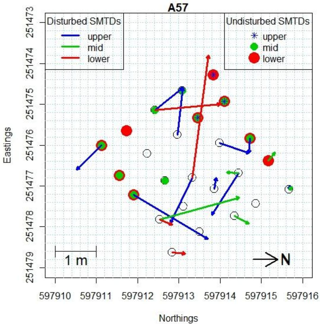
**Figure 6-15: SMTD recovery diagram for stump site A57.** Open circles indicate initial placement positions. Arrows indicate movement path of disturbed SMTDs, coloured by initial burial depth. Circular markers indicate undisturbed SMTD recovery at initial placement site.
