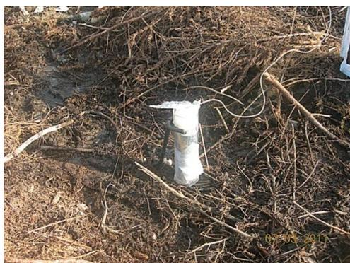
**Figure 4-32: NaI detector in extraction rack.**
