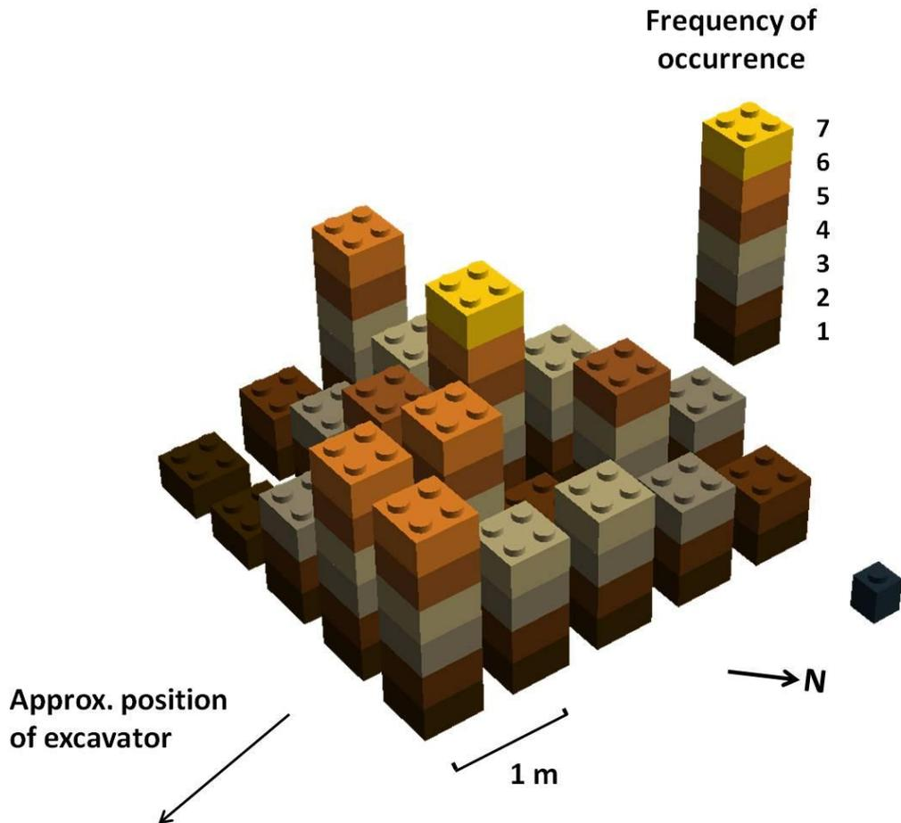
Figure 6-22: Frequency of occurrence of disturbed SMTD at a given placement point from any depth.
