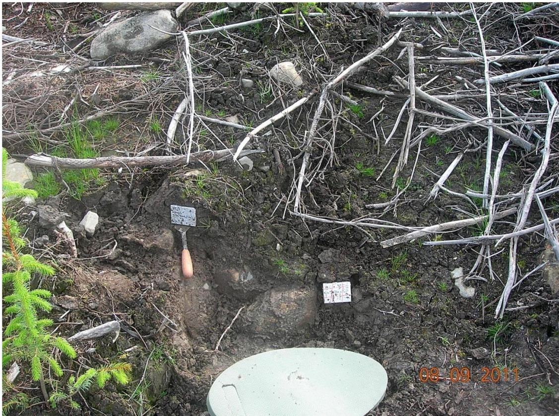
**Figure 5-19: View of surface compaction (sample Trk A on right) by excavator track compared to non-compacted surface on left (Trk B).**
