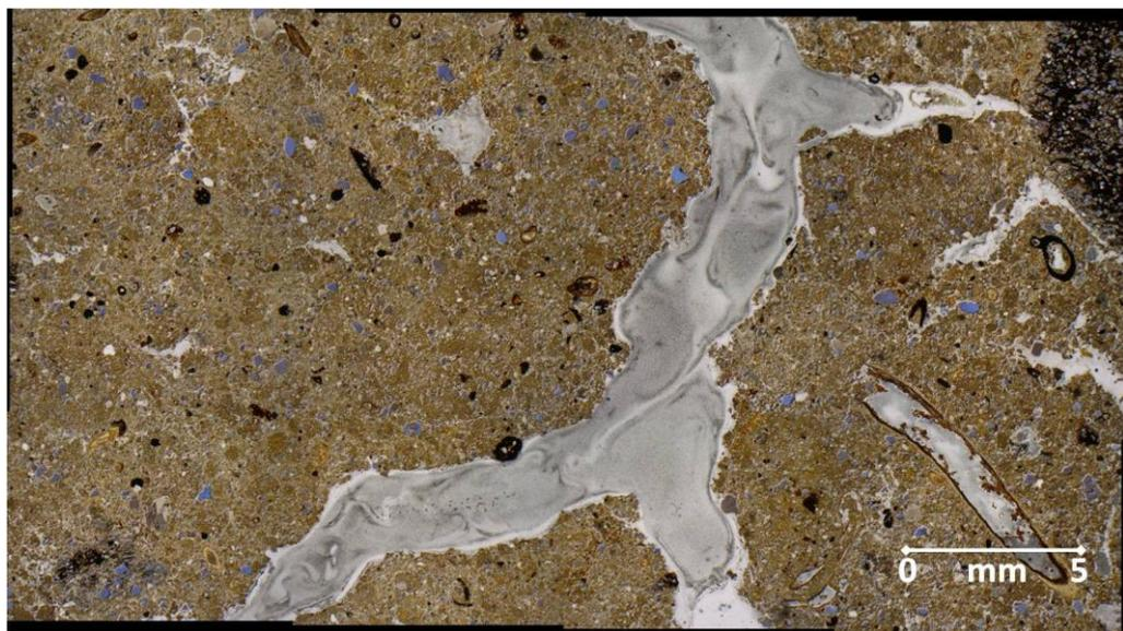
**Figure 5-11: Composite cross polarised and natural light image from sample DS3(B) showing colour contamination in the pore space.**
