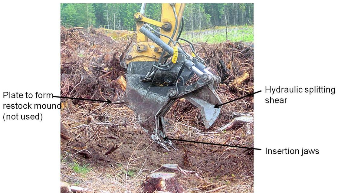
Figure 2-20: Destumping shear head.
