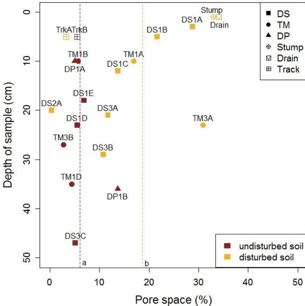
**Figure 5-27: Mean pore space by depth of sample, treatment type and disturbance state for all thin section sample points.** Mean pore space for undisturbed and disturbed soil is shown. Differing alpha subscripts indicate a significant difference at 95% confidence level.
