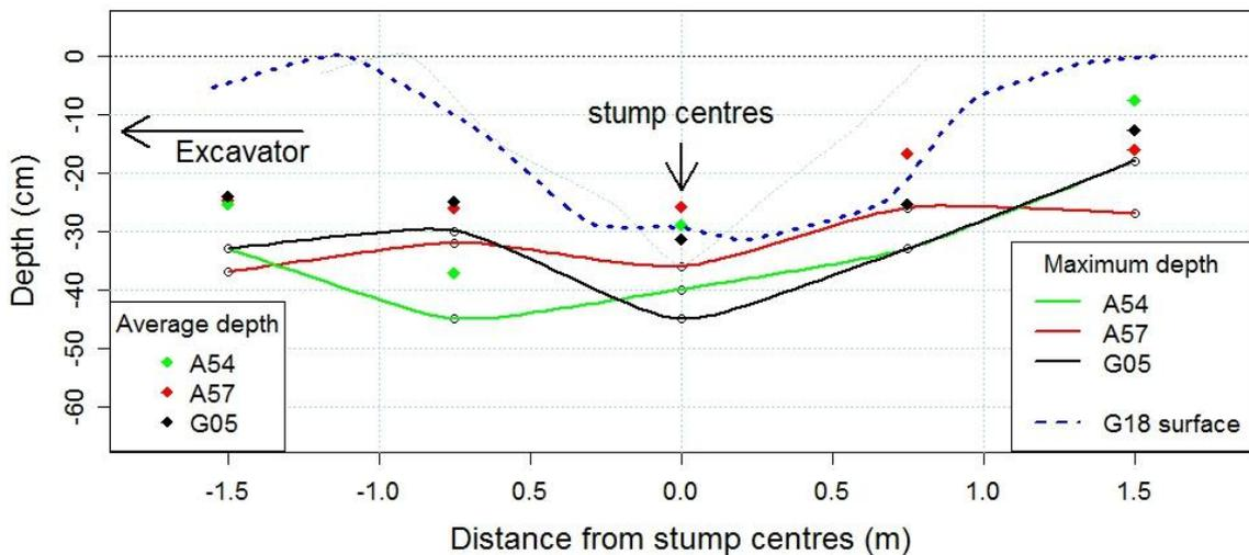
**Figure 6-26: Stump extraction site combined surface survey and disturbance levels.** There is a 2x scale exaggeration on the Y axis. The surface profile from the G18 site major-axis survey has been adjusted to take out hillside slope. Maximum depth values for the three other sites are as highlighted in Table 6-7.
