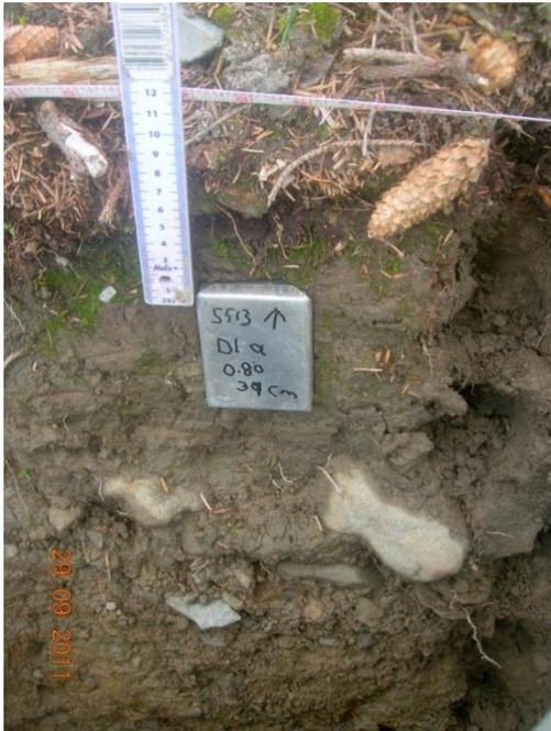
**Figure 5-5: Sample collection for thin section analysis from exposed face of soil inspection trench (DP1).** Evidence of the associated bulk density sampling may be seen at the right of the figure.
