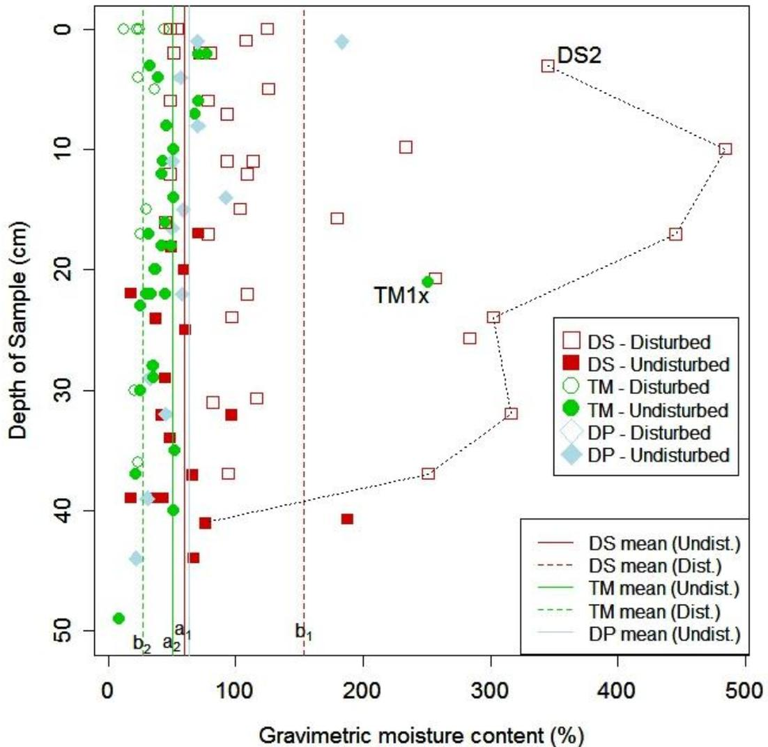
**Figure 5-20: Gravimetric water content results against depth for combined year samples, including mean moisture content by treatment class and disturbance state.** Differing alpha labels against means with the same numeric subscript indicates a significant difference in moisture content between Undisturbed and Disturbed mean values. There are no Disturbed DP samples. The profile of sample points at site DS2 is joined by the dotted line. TM zone outlier point TM1x is identified.
