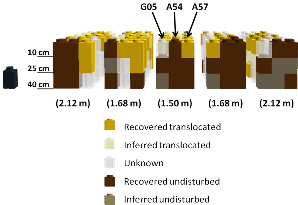
**Figure 6-21: Composite indication of disturbance at “edge” face of stump sites.** Results at each edge placement position is given for the three sites in the order indicated. Depth of placement as indicated. A placement position is inferred as undisturbed if it lies beneath a recovered undisturbed position. The distance to each placement point from the centre of the extracted stump is indicated in parentheses.
