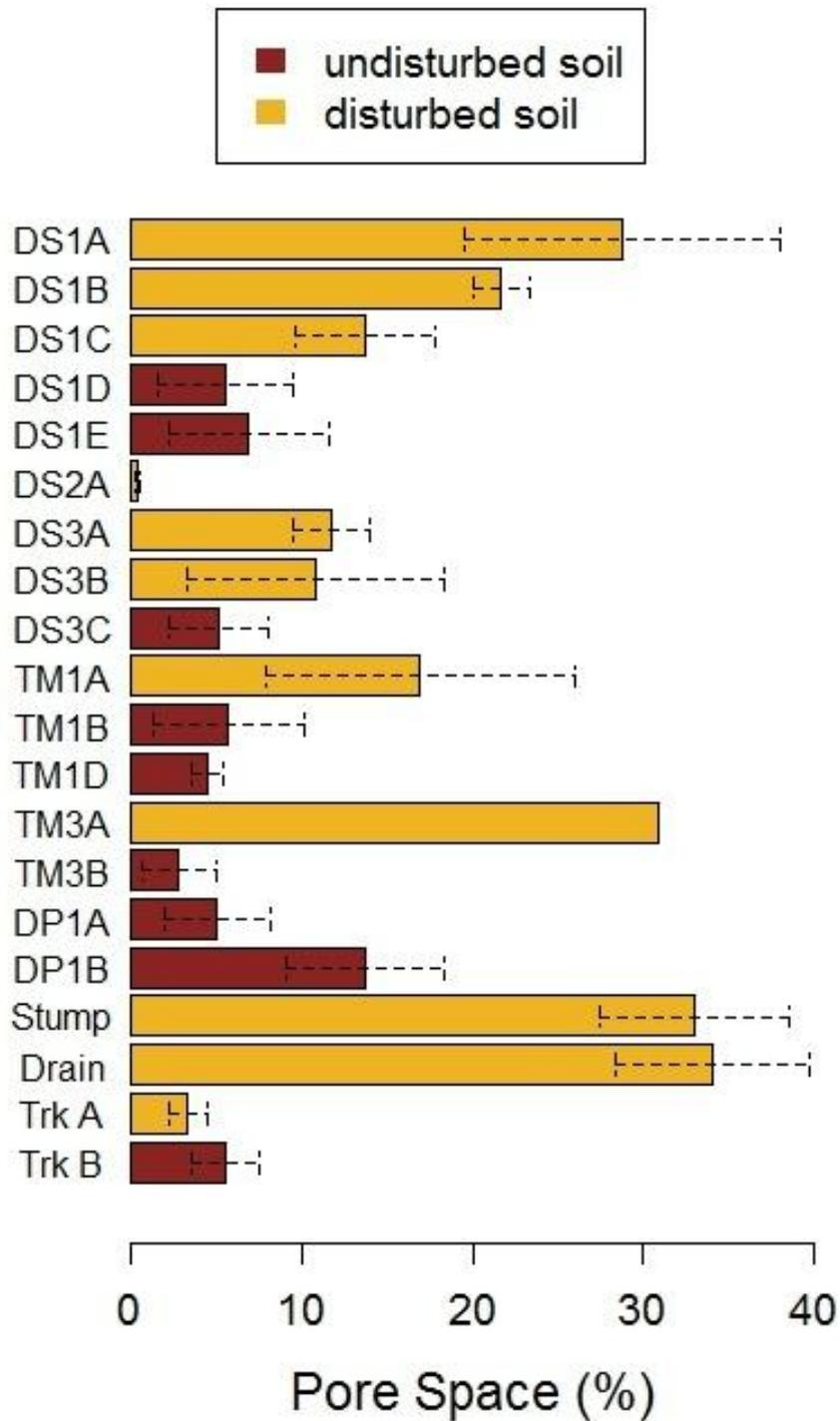
**Figure 5-21: Mean pore space for each thin section slide, differentiated by disturbance state.** One standard deviation is indicated by the dashed line. Only one sample image was taken from TM3A. “Trk A” is a location disturbed by compression of excavator track. “Trk B” is adjacent undisturbed point.
