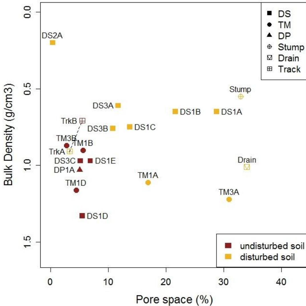
Figure 5-29: Mean pore space against bulk density for all thin section sample points, with disturbance state indicated.
