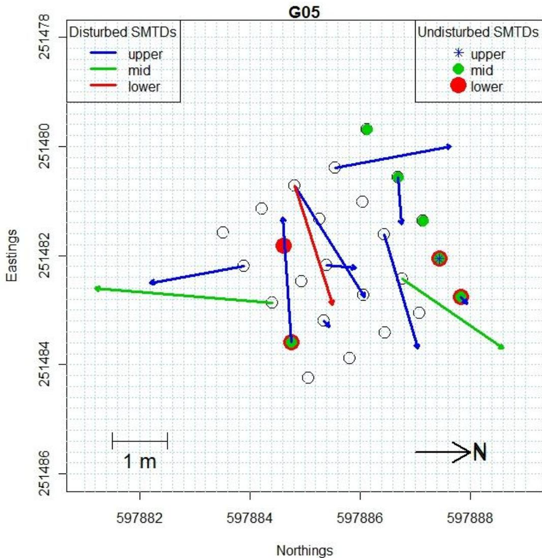
**Figure 6-16: SMTD recovery diagram for stump site G05.** Open circles indicate initial placement positions. Arrows indicate movement path of disturbed SMTDs, coloured by initial burial depth. Circular markers indicate undisturbed SMTD recovery at initial placement site.
