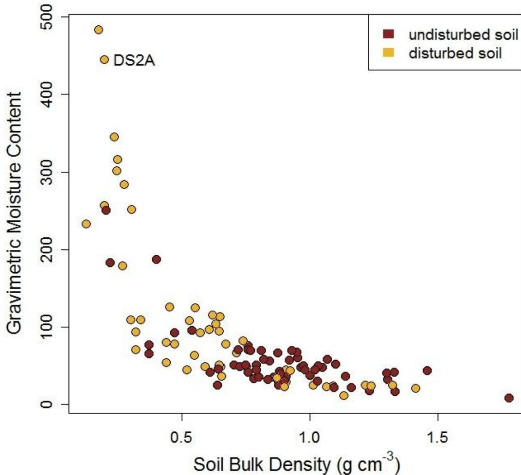
**Figure 5-38: Relationship between gravimetric moisture content and soil bulk density, with DS2A value highlighted.**
