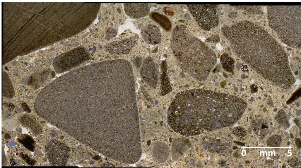
**Figure 5-9: Example of 4x3 mosaiced composite image (undisturbed sample).** Evidence of the stitching process can be seen along the edges to the mosaic.
