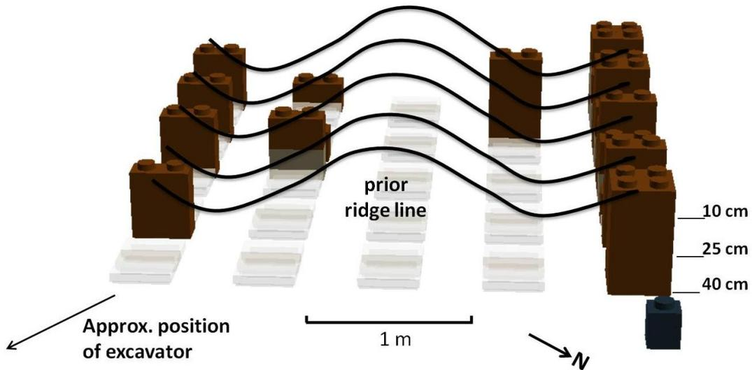
**Figure 6-20: Comparison of pre-destumping ridge line and distribution of undisturbed SMTDs**
