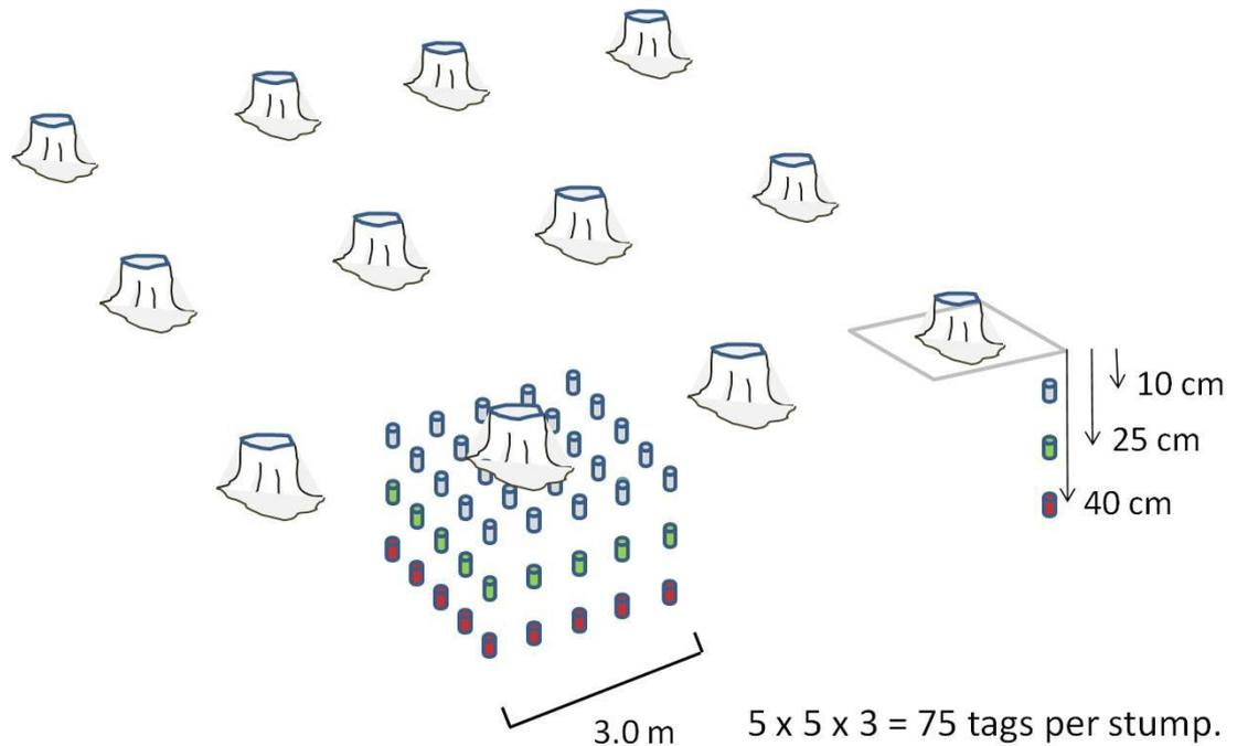
**Figure 6-7: Schematic of SMTD array layout.**
