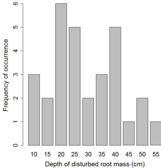
**Figure 6-8: Frequency of stump mass depth measurements (cm) in 30 readings from 10 windthrown trees.**
