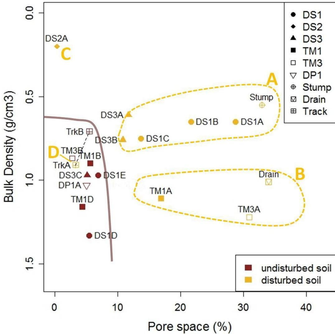
**Figure 5-36: Annotation of Figure 5-29 showing differing effects of disturbance.** The solid brown line encloses the approximate locus of undisturbed points. Dashed outlining and associated identifiers indicate possible groupings of disturbed points.
