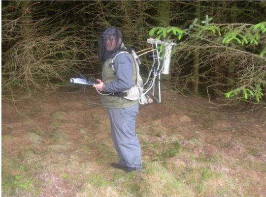
**Figure 4-6: Backpack mounted NaI gamma ray detector for initial  $^{137}\text{Cs}$  survey.**
