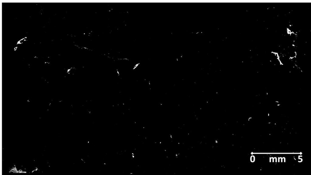
**Figure 5-26: Binary image from DS2, disturbed organic soil at 20 cm depth, pore space 0.4%.**
