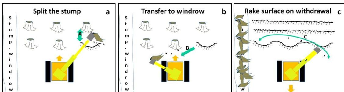
**Figure 6-2: Destumping operational processes.**
