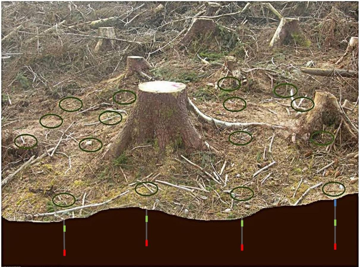
**Figure 6-9: Example of SMTD placement around stump site A54.** The green circles highlight the positions of markers indicating the location of placement columns. The uneven ground surface distorts their relative positions.
