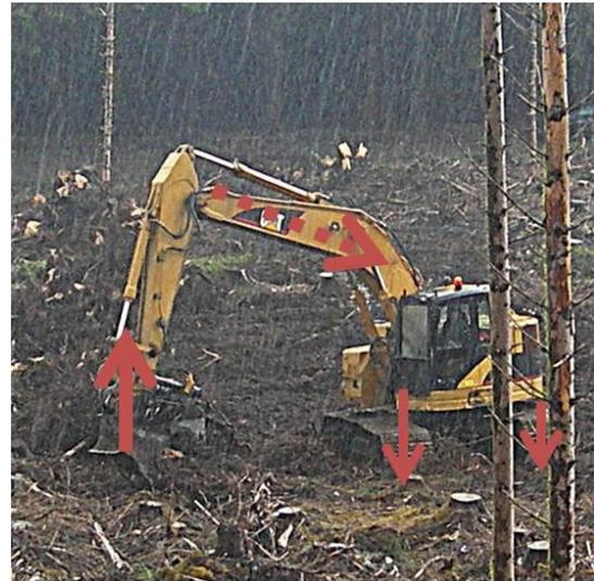
Figure 5-2: Schematic of stump extraction forces.
