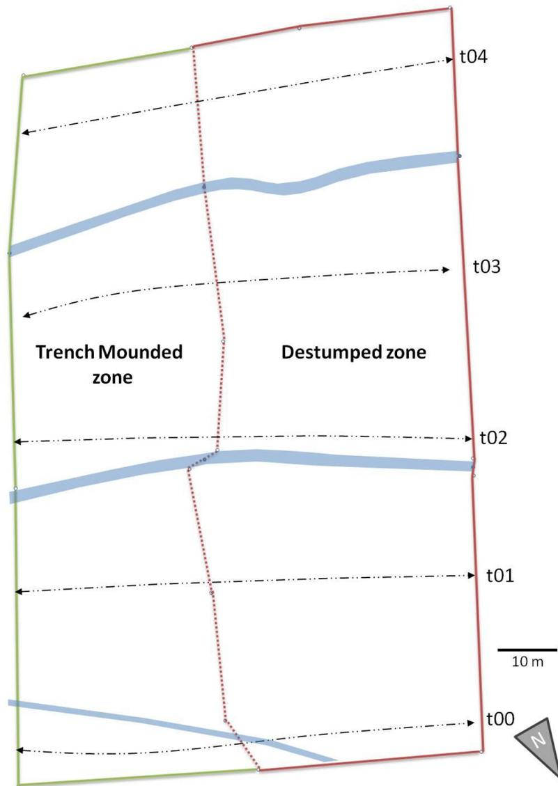
**Figure 2-27: Basic division of research site area between areas that will be destumped and trench mounded.** Dashed lines indicate location of transect lines utilised for visual assessment and radiometric surveys, with transect identifiers included. Blue linear features are drains.
