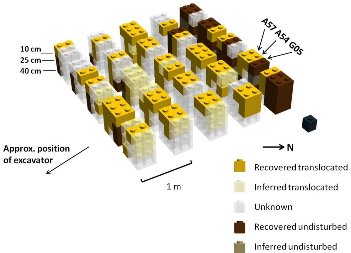
**Figure 6-18: Combined disturbance outcomes for SMTDs at each placement point at all three stump sites.** At each point the results for each of the three destumped sites are arranged in the indicated order. Placement depth from the surface is as indicated. Inferred depths from core samples included where available. Single black indicator brick orients the image as described above.
