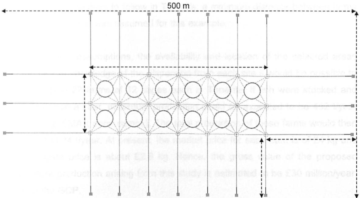
Fig. 7.1: Fish farm composing of 12 polyethylene floating cages of 20 meters in diameter (not to scale). Redrawn with permission from INSEMAR (unpublished data).
