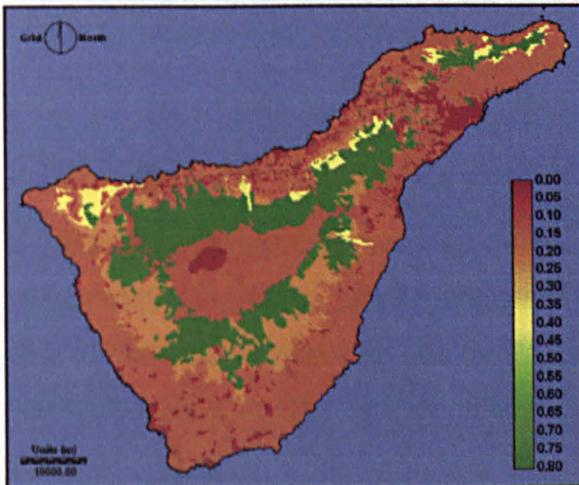
**Fig. 4.72:** Roughness coefficients (Manning's  $n$ ).
