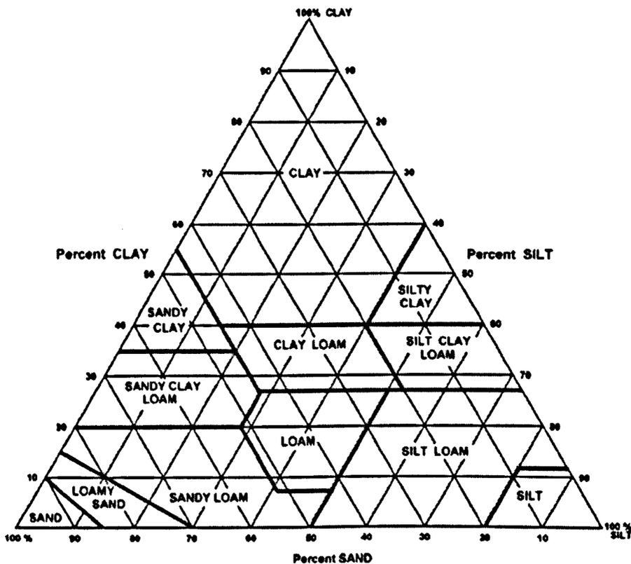
Fig. 3.14: Soil texture classification diagram (from Coche, 1985).
