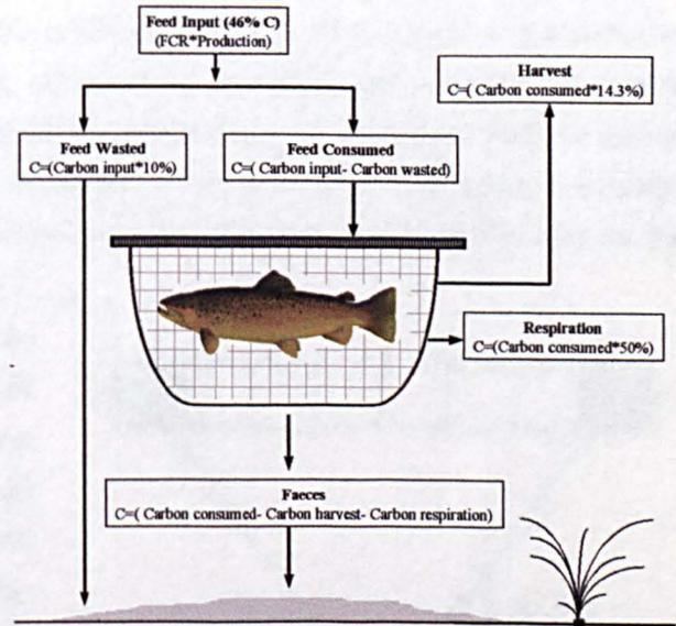
Fig. 1: Mass balance used to calculate carbon wasted from uneaten feed and faecal material in salmon net-pen culture.
