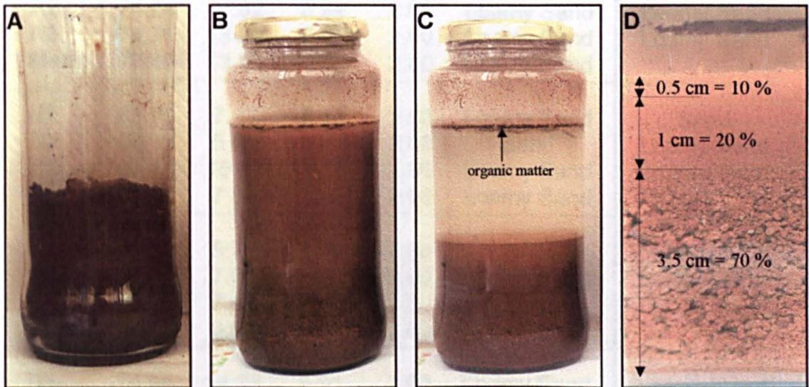
Fig. 3.16: Bottle test steps sequence.
