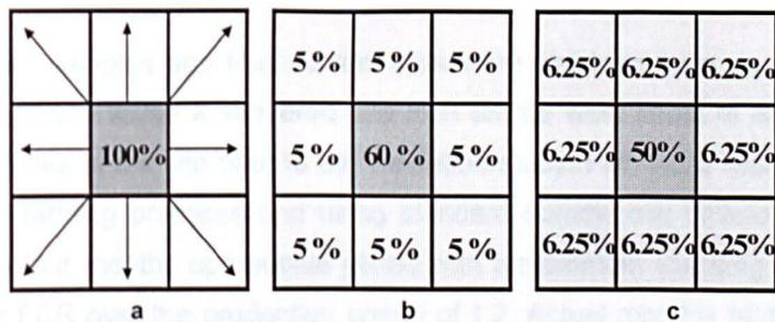
Fig. 3: Sequence of steps involved in "carbon spreading". (a) the original cell as predicted from Gowen's equations, (b) spread of carbon from uneaten feed to surrounding cells, (c) spread of faecal carbon to the surrounding cells.
