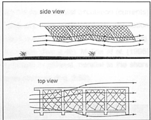
**Fig. 4.43:** Deflection of the net panels due to current (from Beveridge, 1996).
