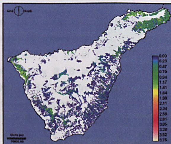
Fig. 4.87: Sediments yield ( $T/100 \text{ m}^2$ ).
