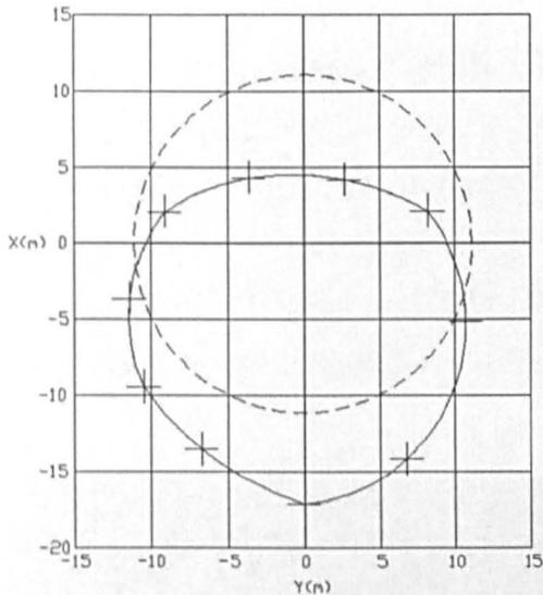
**Fig. 4.42:** Plot of the float ring (polyethylene tubes, PolarCirckel cages) with net in a 0.577 m/s current (Slaattelid, 1990).
