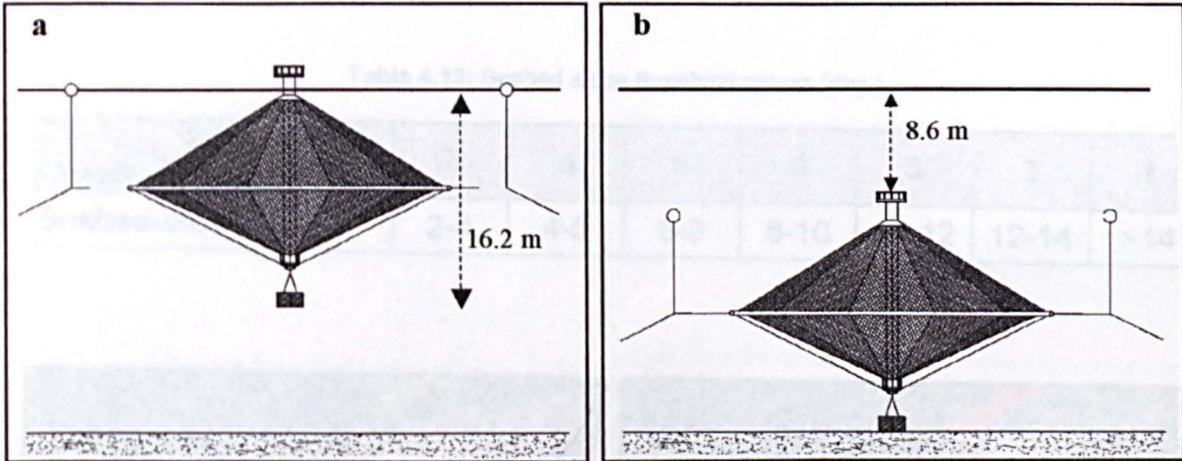
Fig. 4.38: SeaStation® (a) dimension and (b) submergible depth.
