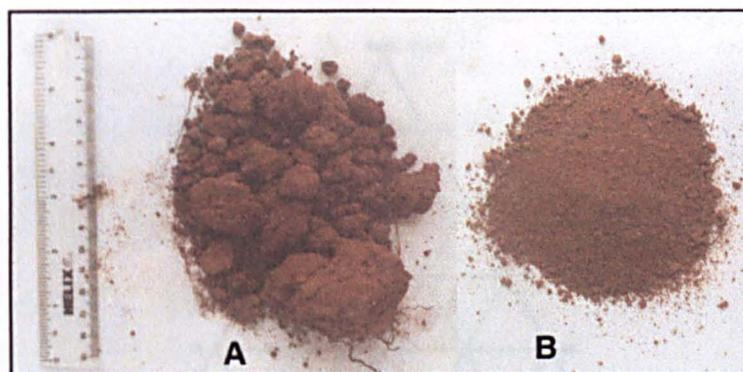
Fig. 3.13: Soil sample before (A) and after (B) after crushing and mixing.
