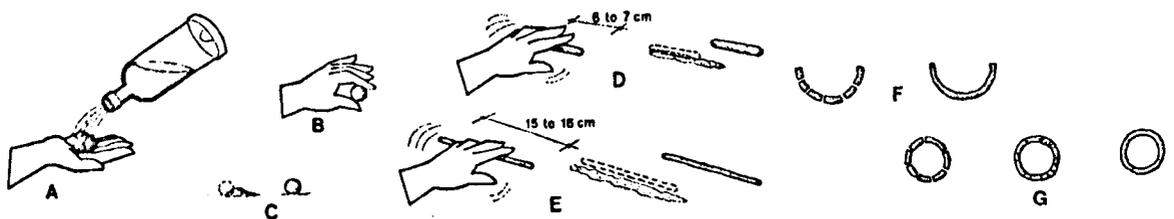
Fig. 3.15: Manipulative test steps sequence (redrawn from FAO, 1985).
