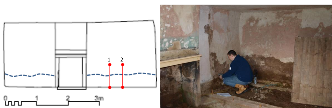
Fig. 9.2. Location of wet/dry boundary and positions of the vertical transects from where XRF measurements were taken on the internal surface of the west gable wall.
