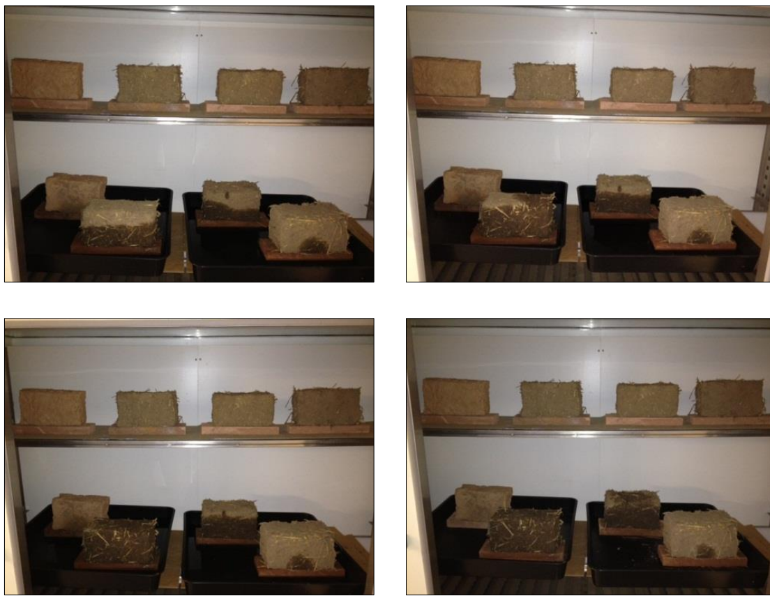
Fig. 6.4. Observations of the earth blocks at weekly intervals (clockwise from top left) through the “Winter-spring 2080s” experimental cycle indicated the same pattern of water uptake as during the baseline conditions, but with reduced intensity. Higher clay content resulted in progressively increased uptake in the experimental blocks over the course of the experiment, whilst the 100 % clay block demonstrated limited water uptake within the first two weeks of the experiment before drying again towards the end of the cycle. It is worth noting the differential rates of water uptake when making comparisons between the two climatic regimes, particularly when considering the variable impacts of temperature on moisture within the walls of the Old Schoolhouse, Cottown, discussed in relation to microwave moisture sensor sampling in Chapter 8.
