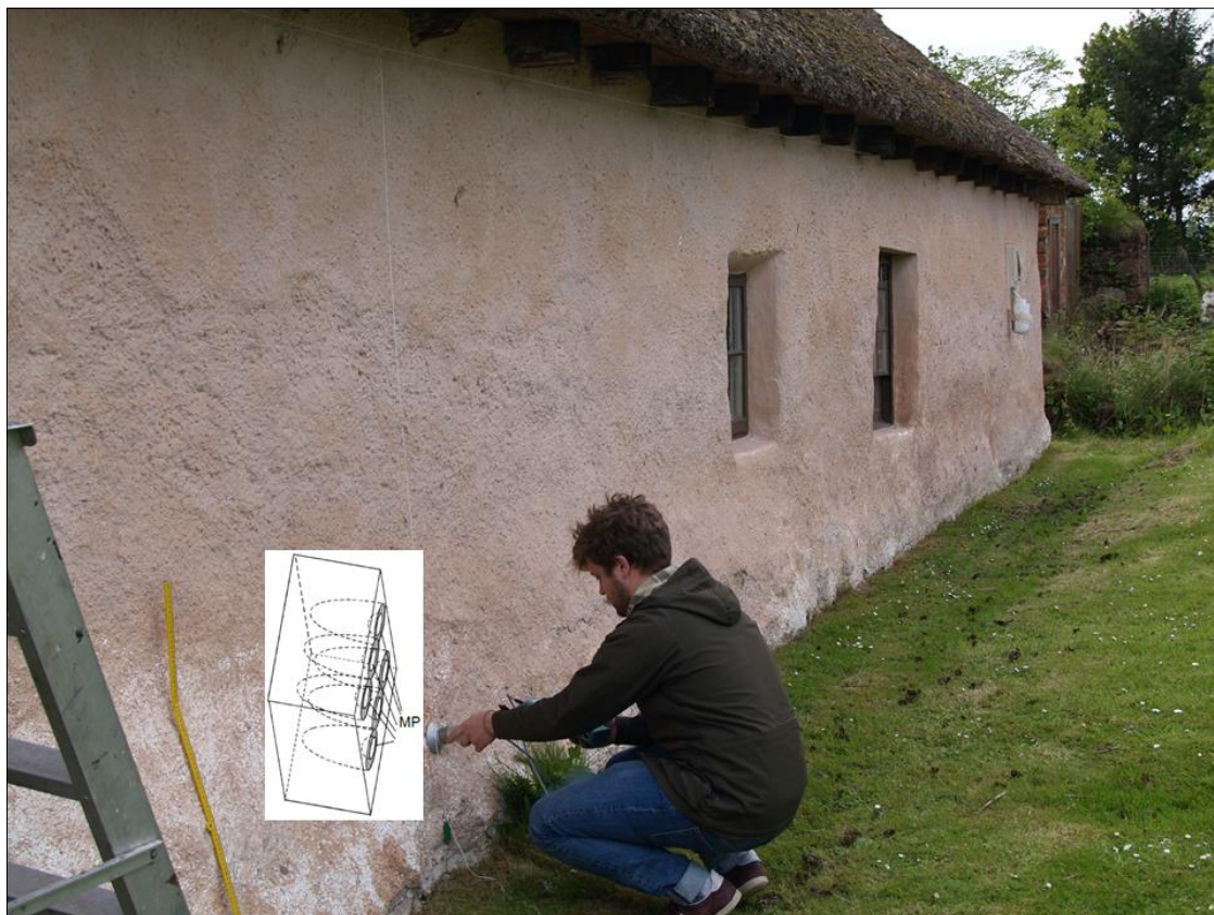
Fig. 8.11. MMS sampling along the north wall of the Old Schoolhouse, Cottown, with diagrammatic example of the “balloons” of microwaves emitted by the moisture meter sensor head.
