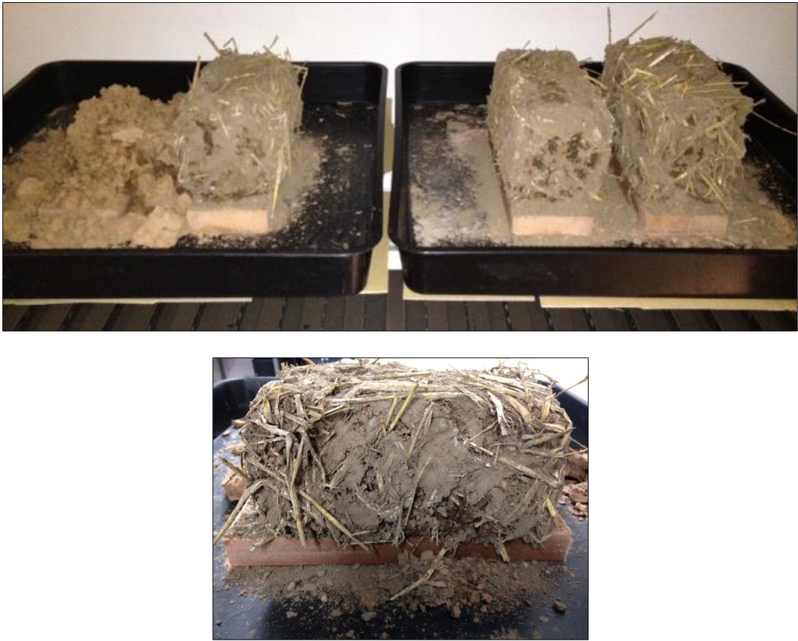
Fig. 6.5. By the end of the “Freeze-thaw baseline” experimental cycle the 100% clay block had completely failed and the admixture blocks exhibited surface damage whereby the outer material had dissociated and dried out.
