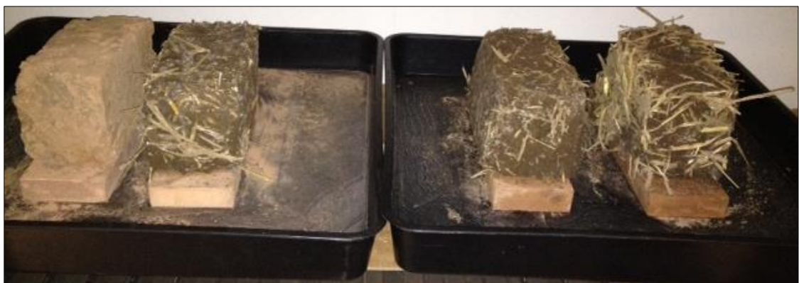
Fig. 6.6. In contrast, all blocks retained their cohesion after being subjected to the “Freeze-thaw 2080s” experimental cycle and the lack of surface deterioration is indicated by the uniform retention of moisture across the admixture blocks.
