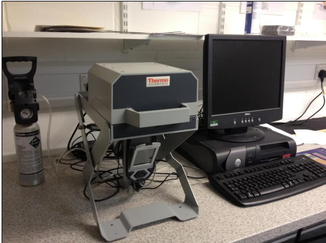
Fig. 3.14. Niton XL3t-Goldd+ X-ray fluorescence analyser used with helium purging (left) to enhance signal quality
