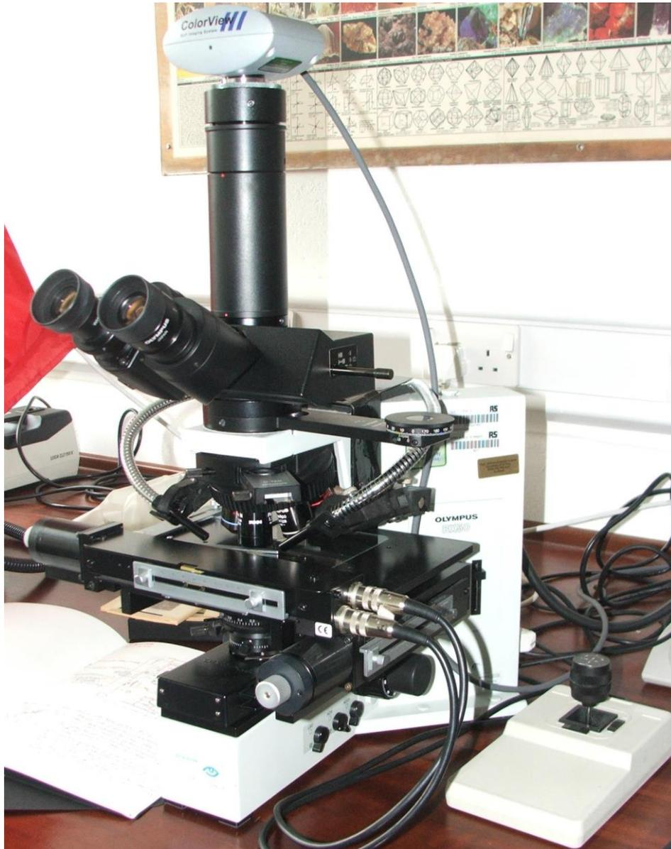
Fig. 3.13. Olympus BX-50 petrological polarizing microscope, automated stage and software-controlled microscope camera used for thin section image analysis
