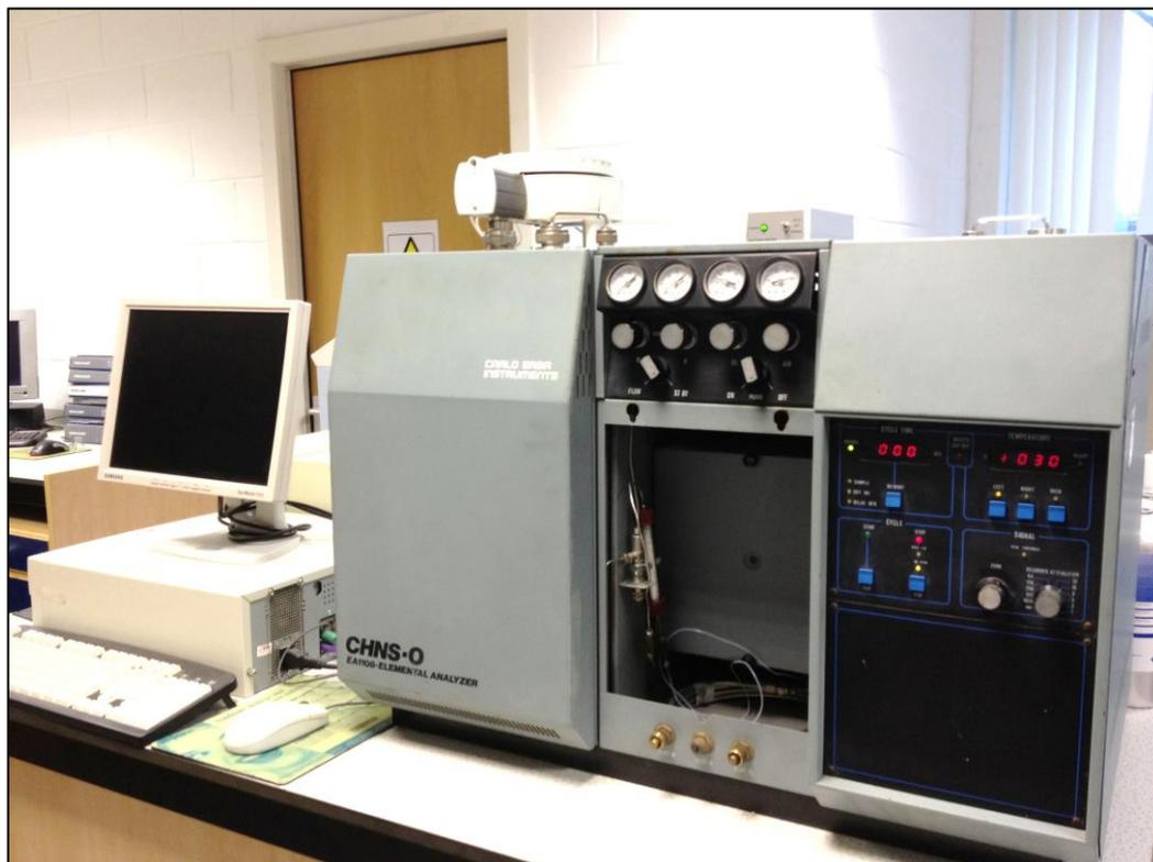
Fig. 3.16. Carlo Erba EA1108 CHNS-O elemental micro-analyser used to determine the total carbon and nitrogen of soil samples
