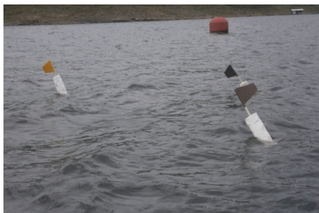
Figure 12: Drogues deployed in Lake Volta
