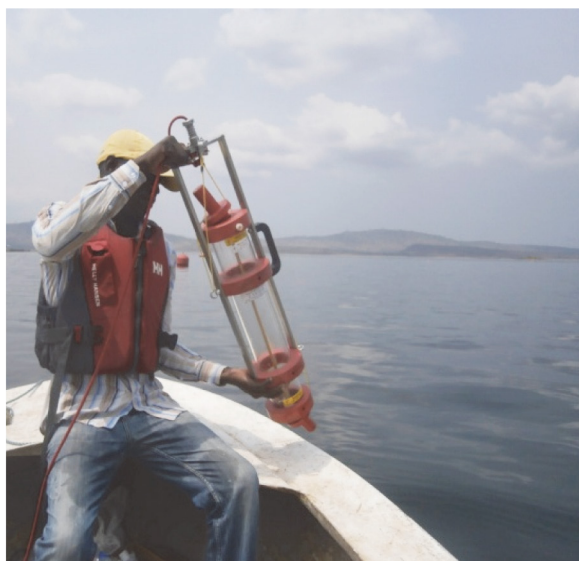
Figure 13: Collecting water samples with a Van Dorn water sampler
