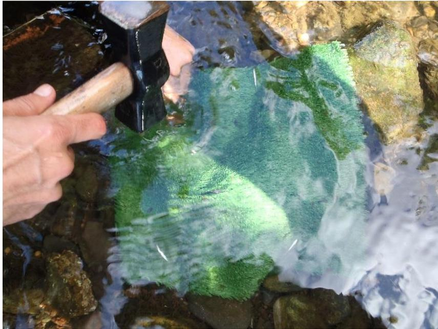
Fig 4.6 Locating a sediment collection mat on the stream bed.
