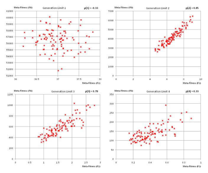
Figure 3: All 100 DE configurations plotted by meta-fitness on function F1 and meta-fitness on function F6, for generation limit of 1 (top-left,  $\rho = -0.33$ ), 2 (top-right,  $\rho = 0.85$ ), 3 (bottom-left,  $\rho = 0.78$ ), and 4 (bottom-right,  $\rho = 0.33$ ). Note that the scales on both axes decreases with generation, as the algorithms advance.
