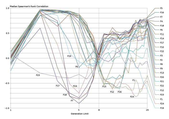
Figure 4: The median Spearman's rank correlation by generation (log-x) limit on all BBOB benchmarks of dimension 10, for DE using a parameter sweep around  $\theta = (F = 0.3, CR = 0.9)$ . Generation 8 has been highlighted as the crossing point.
