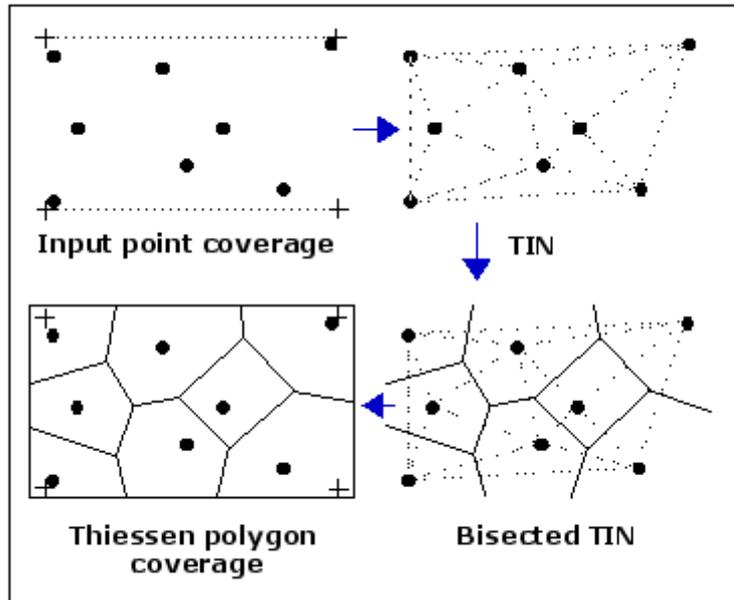
**Figure 5.14.** Given a set of random points a TIN (triangulated irregular network) are generated then perpendicular bisectors of the lines connecting the points are traced in order to derive the Thiessen polygons (Source: ArcGIS help-on-line).
