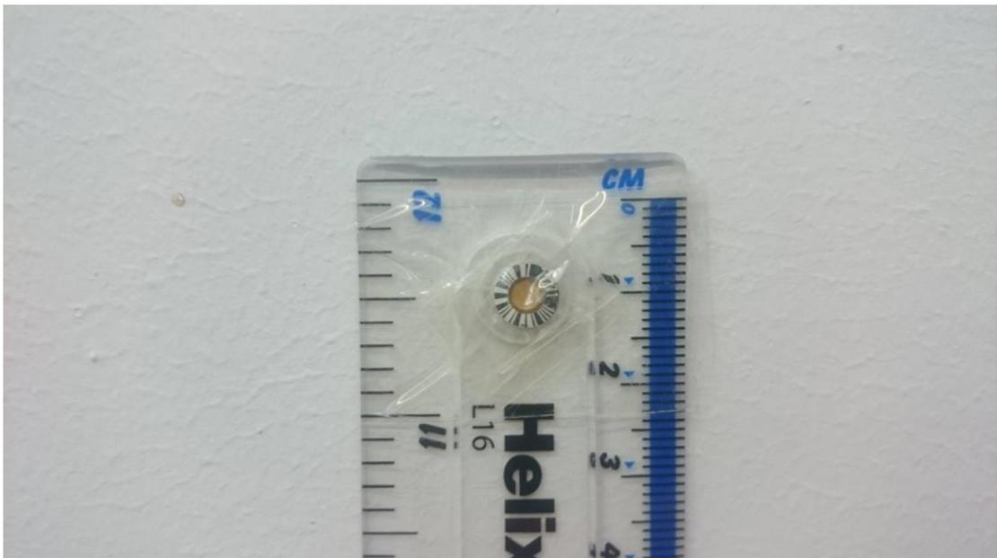
*Figure 3.4 Perspex ruler with inserted TLD to shield to allow contribution from beta and gamma radiation to be buried into the ground. TLD mounted at 10 and 30 cm.*
