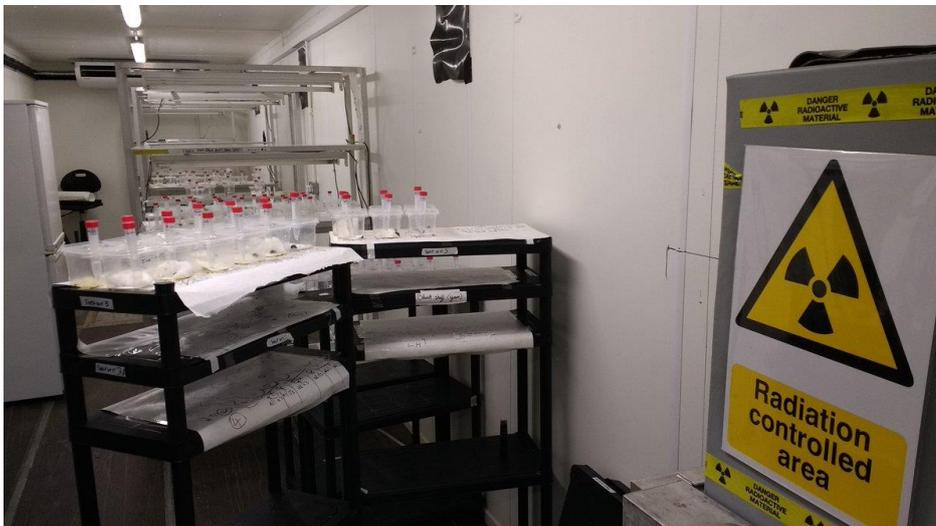
*Figure 4.3 Radiation facility at Stirling University. Individual bumblebees in their housing were randomly assigned a radiation treatment. Different radiation dose rates generated by calculating distance from the  $^{137}\text{Cs}$  source verified using an electronic personal dosimeter.*
