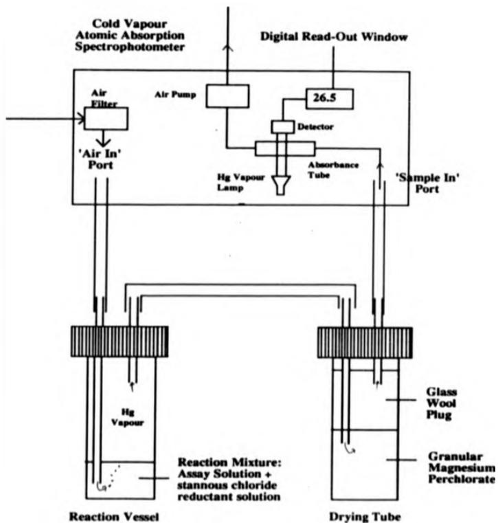
**Fig. 2.10** Cold Vapour Atomic Absorption Spectrophotometry system for determination of total mercury.
