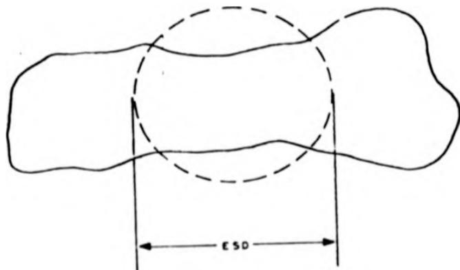
Fig 2.6 Equivalent Spherical Diameter (ESD) (reproduced from Coulter manual).
