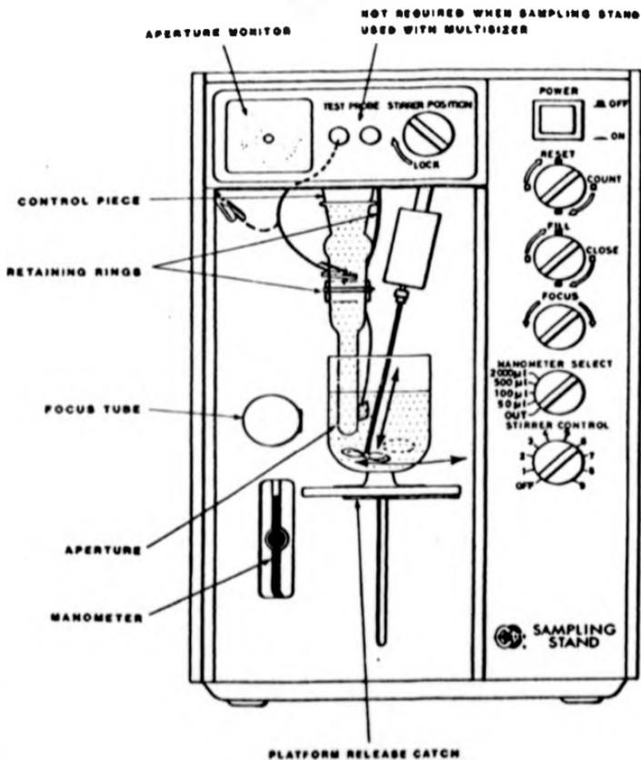
Fig. 2.3 Sampling stand front view (reproduced from Coulter manual)
