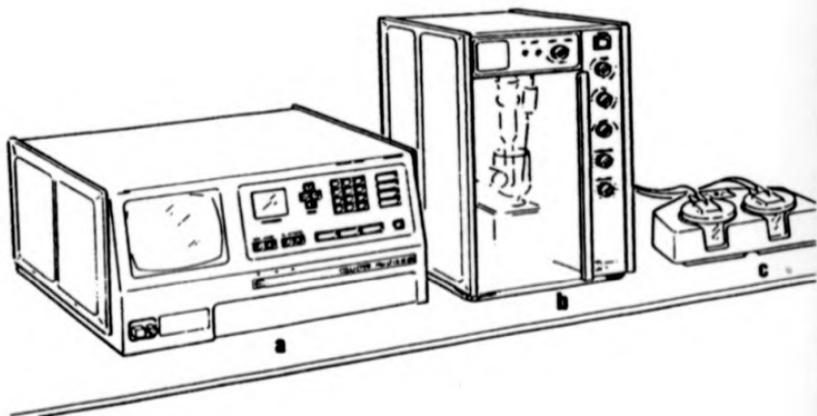
Fig. 2.1 The Coulter Multisizer (a) Multisizer; (b) sampling stand; (c) vacuum control unit (reproduced from Coulter manual)
