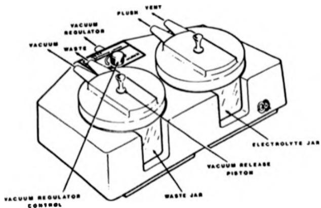
Fig. 2.4 Vacuum control unit (reproduced from Coulter manual)
