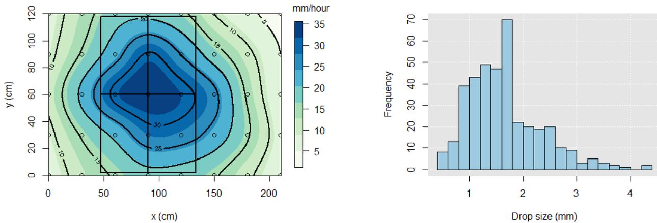
**Figure 5.2.** The left plot shows the spatial variation of simulated rain within the rainfall simulator; boxes indicate placement of soil-runoff boxes and the circles indicate the placement of rainfall collection pots. The distribution of droplet size is shown in the right hand figure.
