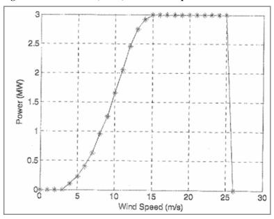
Figure 4.18 Vestas V90 (3MW) wind turbine power curve.
