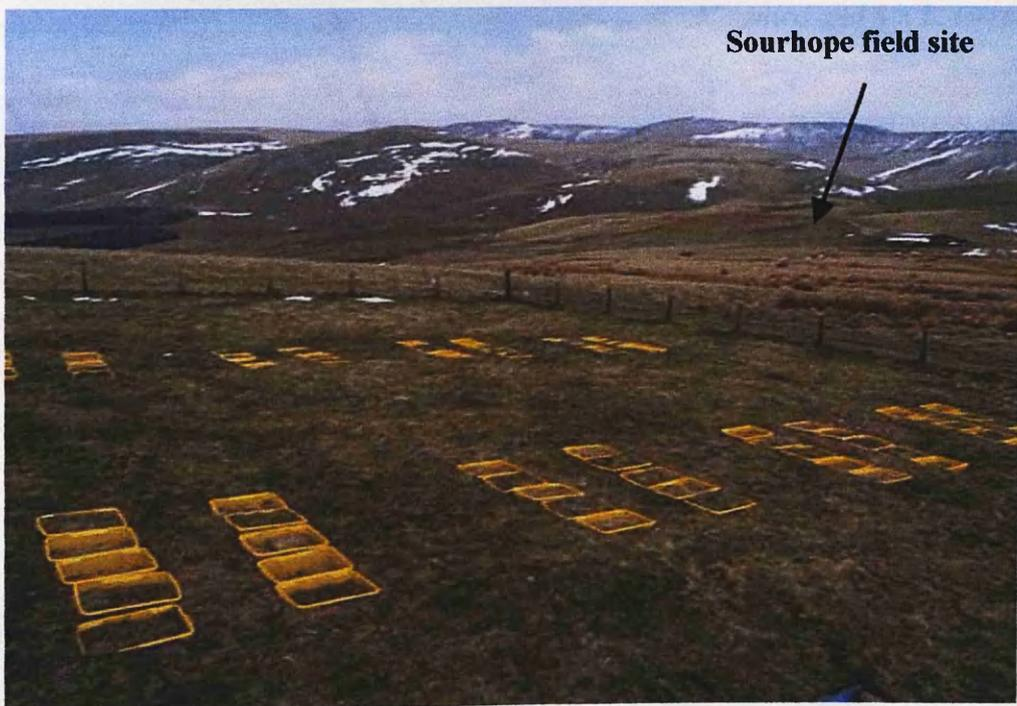
**Figure 2.7 Mesocosm site showing plastic boxes in trenches prior to earthworm inoculation, with Sourhope field site in the background.**
