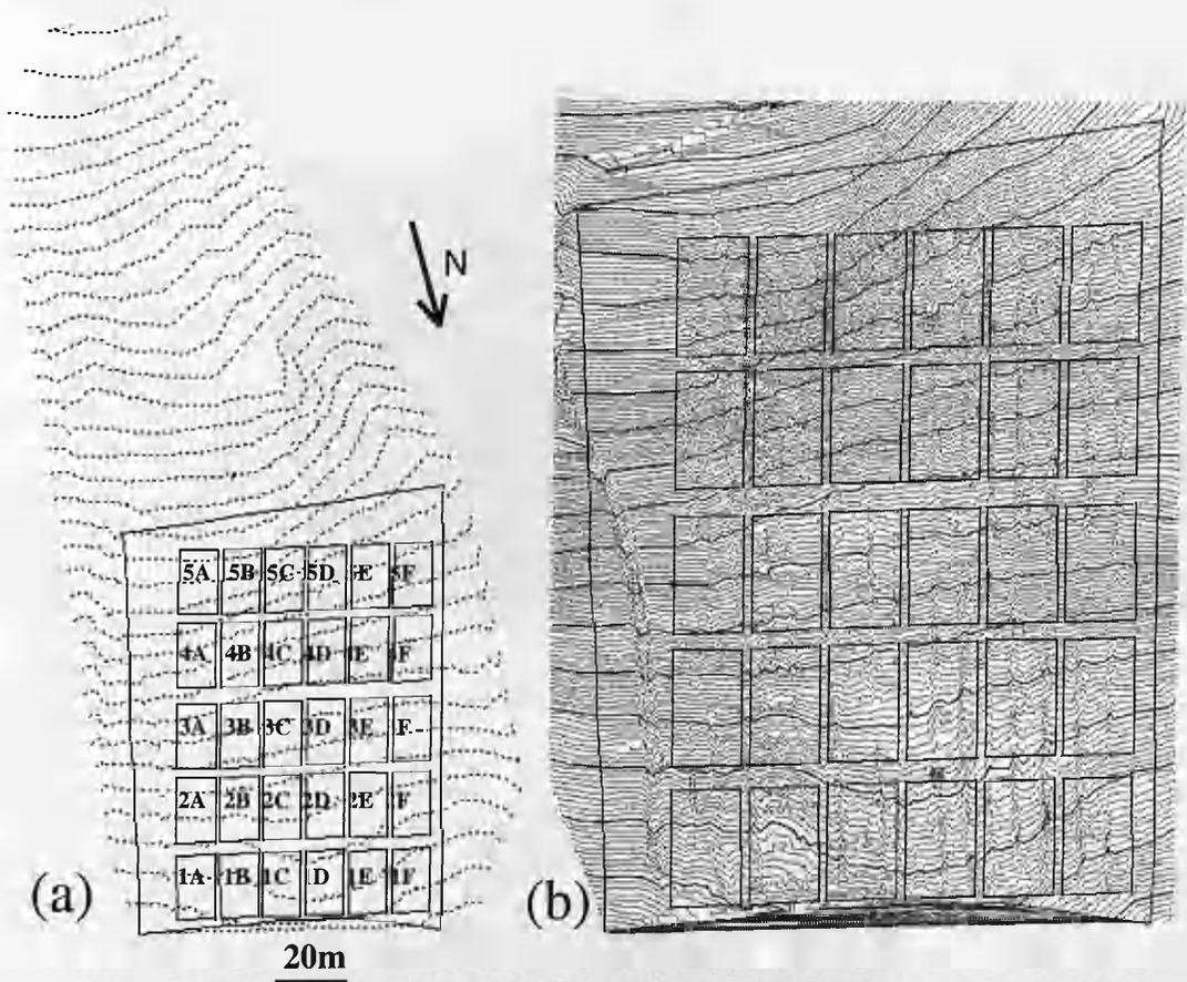
**Figure 2.4** Topography of the Sourhope field site showing a) topographic context of the fenced area and b) detailed topography within the fenced area. Major contours 1m, minor contours 0.1m. Major plot boundaries are also shown. (Whelan *et al.*, Submitted).
