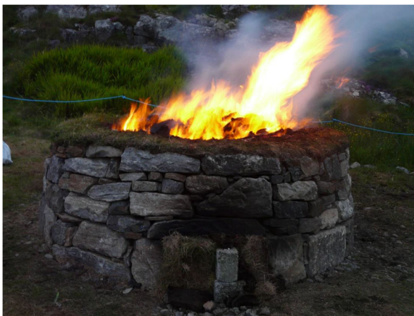
Fig. 2 A replica limekiln constructed on the Isle of Barra in 2014 and fired using the mixed-feed technique. This circular kiln was constructed and charged with alternate layers of peat and shell; relict evidence for which was noted in multiple phases of the nearby Castle Kisimul (Thacker 2014; Ostrich 2015, 416–7). Photograph: M. Thacker
