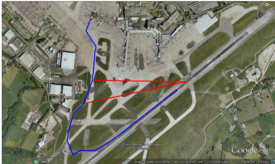
Figure 4: Example of cleaning time-coordinates on a movement at Manchester Airport. The original track is in red, the cleaned track is in blue (blue overlaying red for most of the track). One coordinate in the raw data was an outlier, located on the runway, which was successfully removed.
