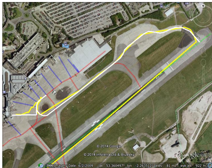
Figure 11: The final snapped path (white), overlaid on the raw flight track to be snapped (yellow), taxiways (red), stands (blue) and runway (green).
