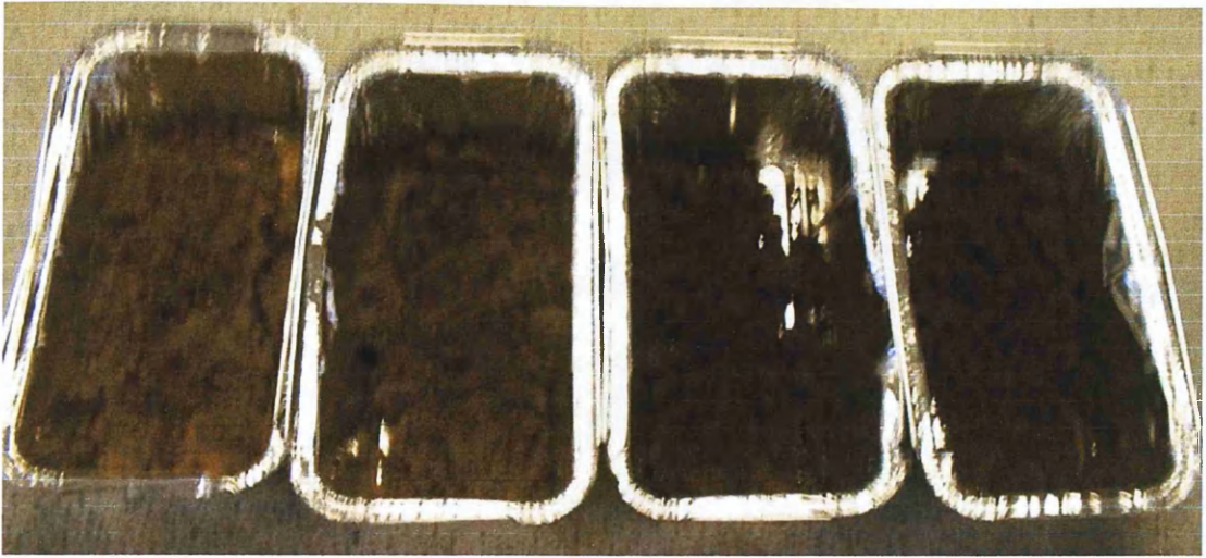
Figure 4.22. Visual comparison of soil colour changes with depth for the deposit 3 at 0-5, 5-10, 10-15, 15-20 cm depths, dried at 30°C.
