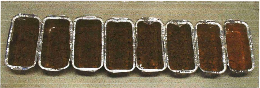
Figure 4.16. Visual comparison of soil colour changes with depth for core 10 at 0-5, 5-10, 10-15, 15-20, 20-25, 25-30, 30-35, 35-40 cm depths, dried at 30°C.
