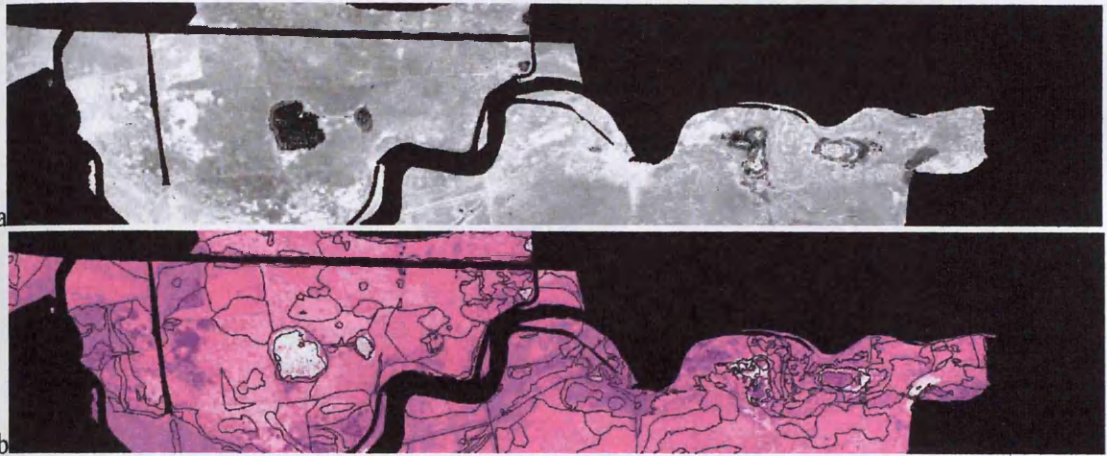
Figure 6:21 Position of red edge calculated for CASI 91 a) Raw Results b) Results grouped via K-Means Classification into 10 classes
