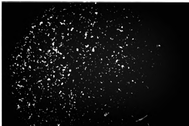
FIGURE 4.6 (b) Photomicrograph showing the mosaic texture of the smectic B phase of copolymer 1b (Magnification x 100).
