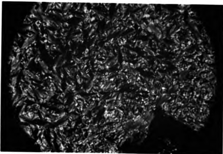
FIGURE 2.4 Photomicrograph of a typical smectic A fanned focal-conic texture (magnification \times 100 ).
