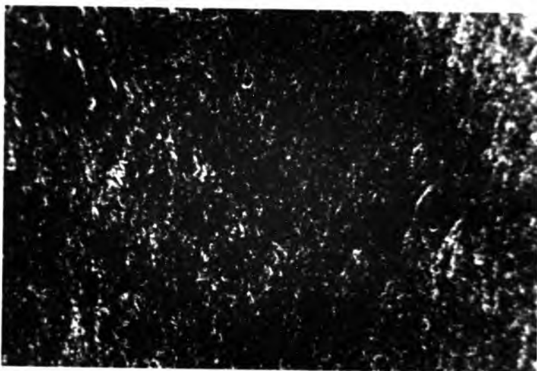
FIGURE 5.12 (b) Photomicrograph of the planar texture of the cholesteric phase of copolymer 4c after annealing for 12 hours (Magnification x 100).
