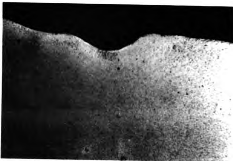
FIGURE 6.20 (c) Photomicrograph of the planar texture of copolymer 8a at 96°C exhibiting the reflection of yellow light (Magnification x 200).
