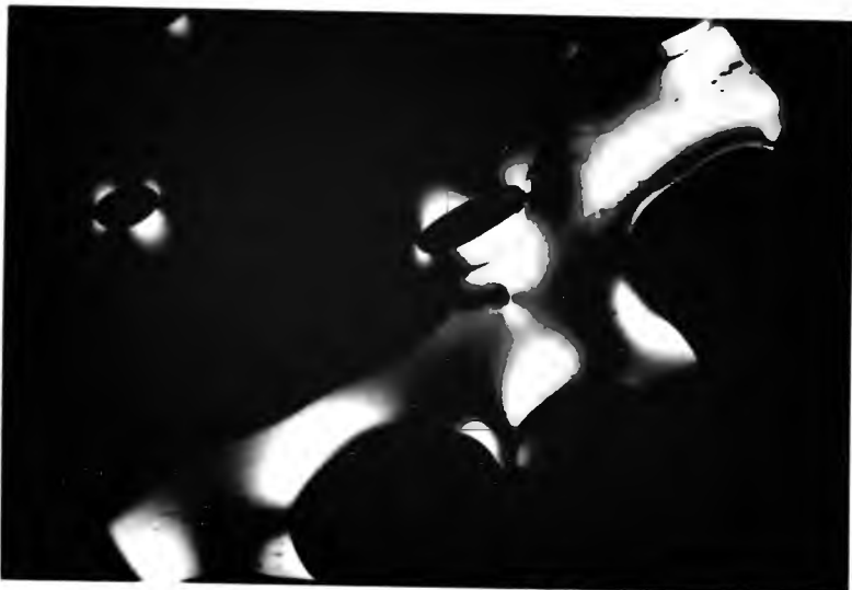
FIGURE 4.17 (a) Photomicrograph of polymer 3c showing the planar homogeneous texture and homeotropic regions (Magnification x 200).
