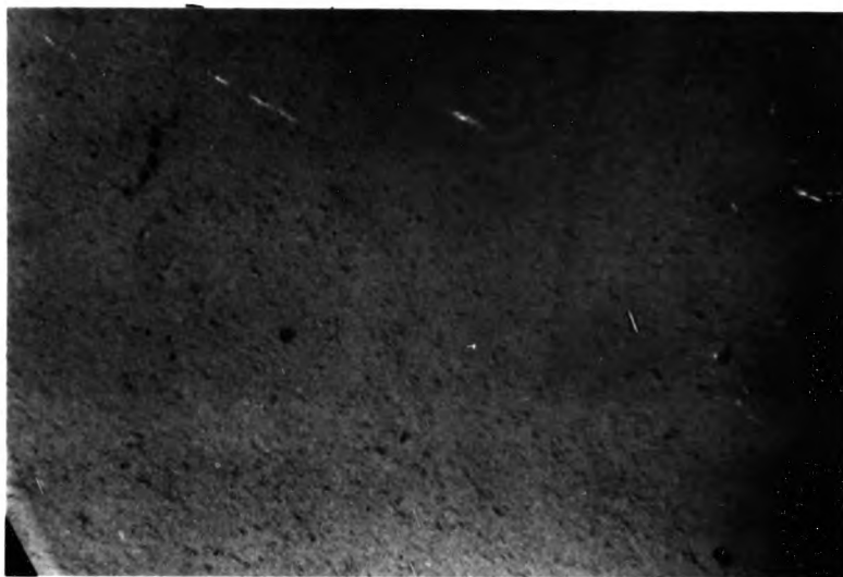
FIGURE 6.22 (a) Photomicrograph of the planar texture of copolymer 8c at 83°C exhibiting the reflection of blue light (Magnification x 100).
