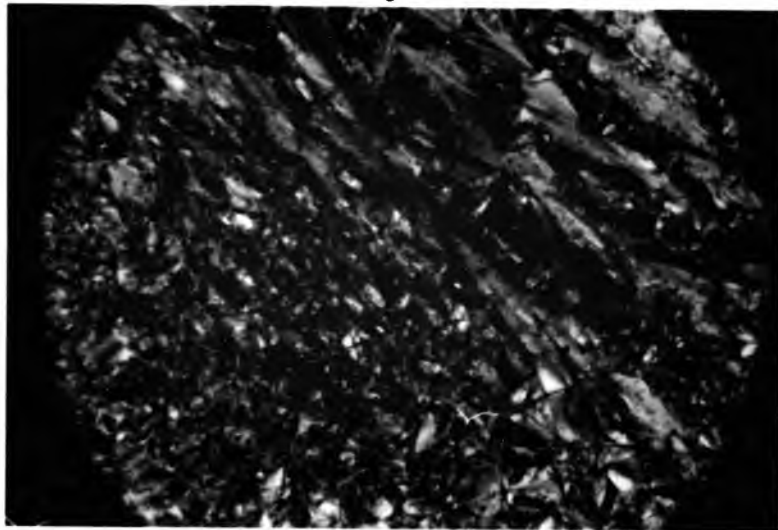
FIGURE 4.12 (b) Photomicrograph of the smectic A phase of polymer 2a, showing focal-conic fanned domains (top right hand side) and less well formed fanned domains (lower left hand side) (Magnification x 200).
