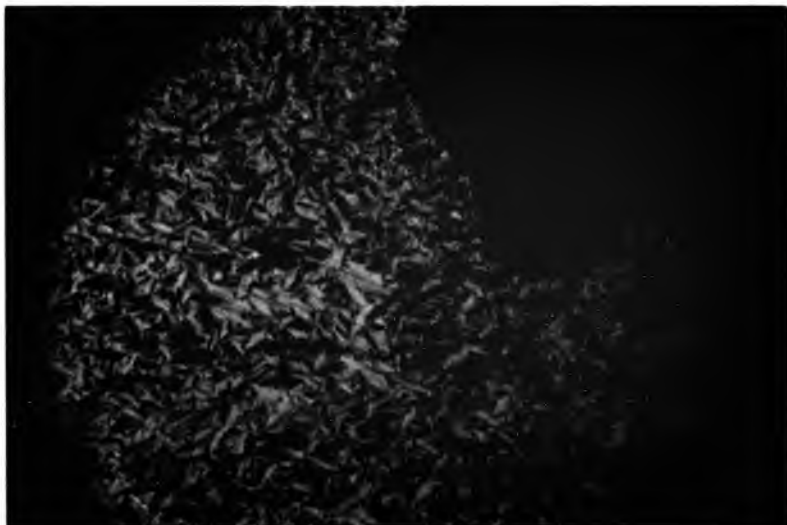
FIGURE 4.6 (a) Photomicrograph showing the fanned focal-conic texture with transition bars at the smectic A to smectic B transition of copolymer 1b (Magnification x 100).
