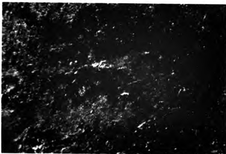
FIGURE 5.12 (a) Photomicrograph of the planar texture of the cholesteric phase of copolymer 4c before annealing (Magnification x 100).
