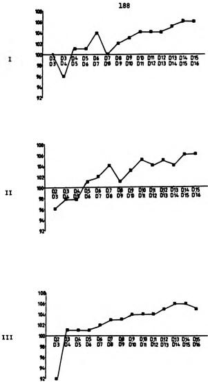
FIGURE 4.4 Diagrams of increment values of DCBEs for programme rate of 3 deg min<sup>-1</sup> on CPSil5-CB column. I) Starting temp 80°C II) Starting temp 100°C III) Starting temp 120°C
