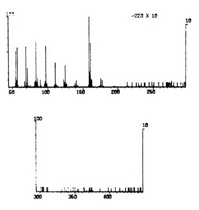
FIGURE 3.8 Mass spectrum of 2,4-Dichlorobenzyl Tetradecyl Ether.
