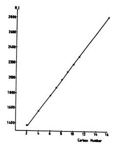
FIGURE 3.13 Graph of retention index versus carbon number of alkyl chain of DCBEs described in Section 3.3.2.
