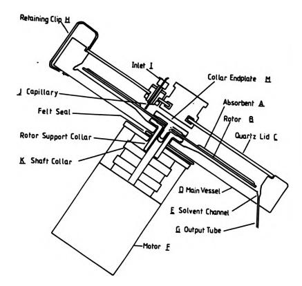
FIGURE 4.3 Schematic diagram of Chromatotron.
