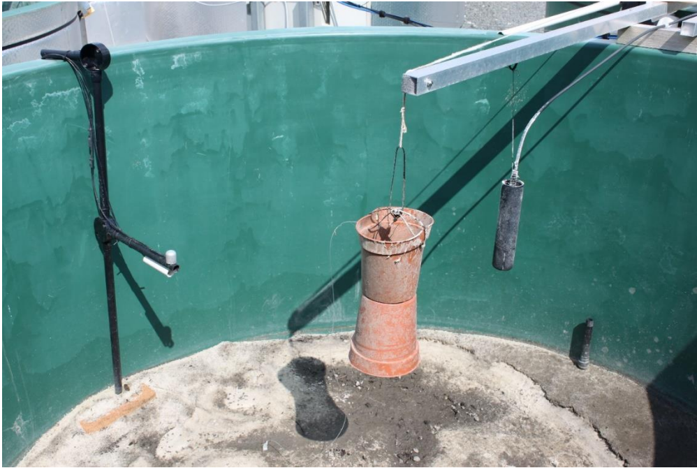
Fig. S3.4 Image showing mixers which are suspended in the middle of each mesocosm and move up and down to allow disruption of thermal stratification. The top and bottom of the mixers are hollow to increase mixing.
