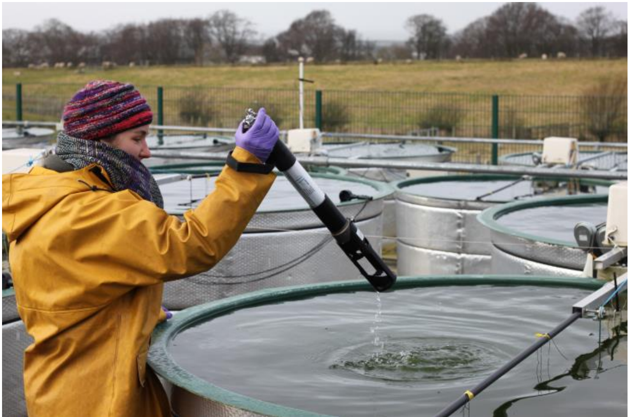
Fig. 3.1 Using a submersible fluorometer (bbe Moldaenke AlgaeTorch) to measure the fluorescence of phycocyanin, a quantitative biomarker for cyanobacteria.
