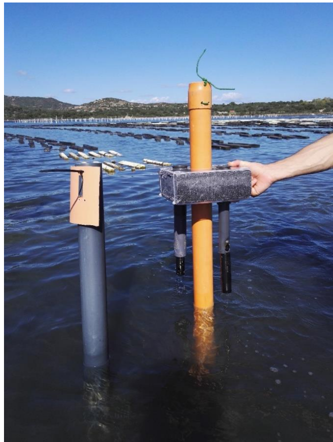
Figure 3.3: Floating station with attach, temperature, salinity and dissolved oxygen data loggers.
