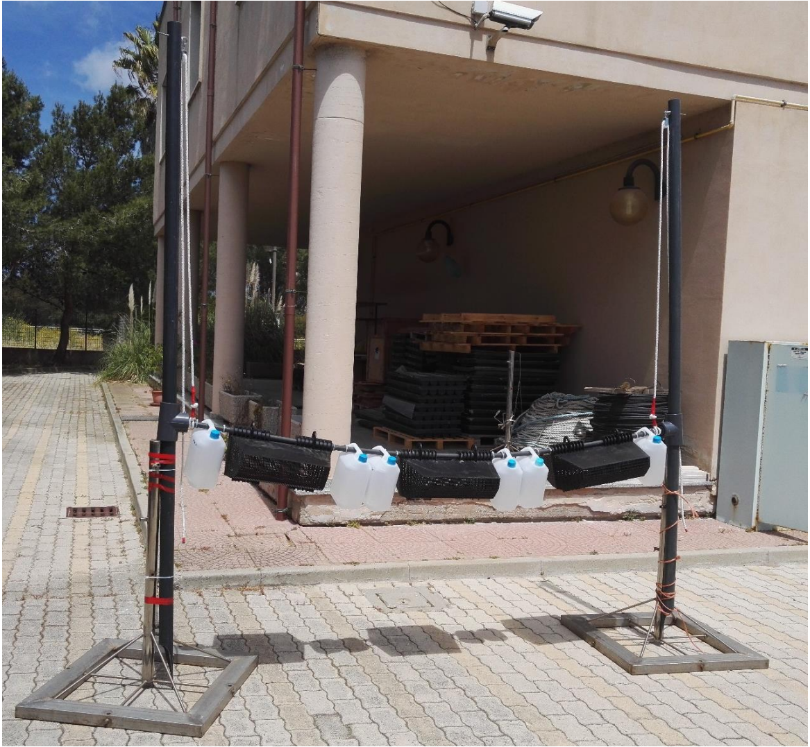
Figure 6.1: The structure in the picture was made with the aim to keep the attached Ortac units on the water surface, but at the same time to give the possibility to keep them out of the water simulating the ocean tides.
