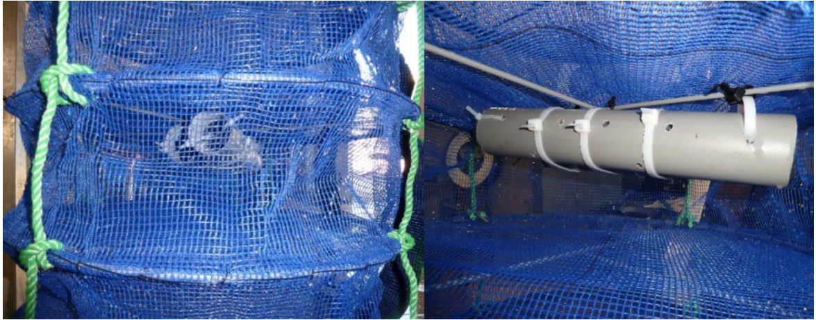
Figure 3.4: Data logger in the Santa Gilla lagoon. All of these were inserted in a pvc pipe and attached inside a lantern.
