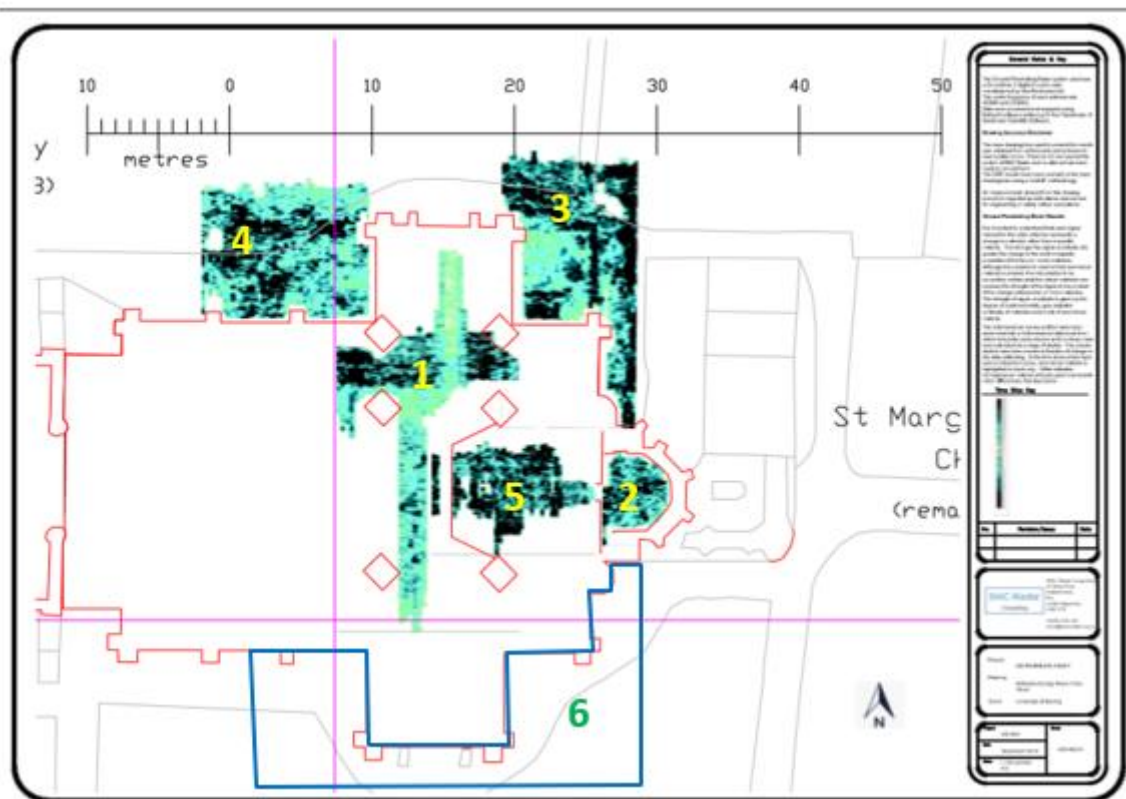
Fig 4: Composite GPR scan areas of the overbuilt Dunfermline Abbey choir, 2016 [1, 2], 2017 [3, 4, 5] and 2019 [6] [© Atlas Geophysical]
