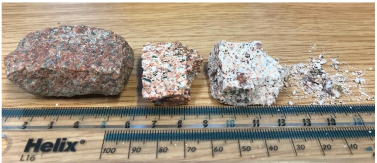
Figure 41: Progression of the dehydration and friability of granite as temperature increases between 750 and 1250°C.
