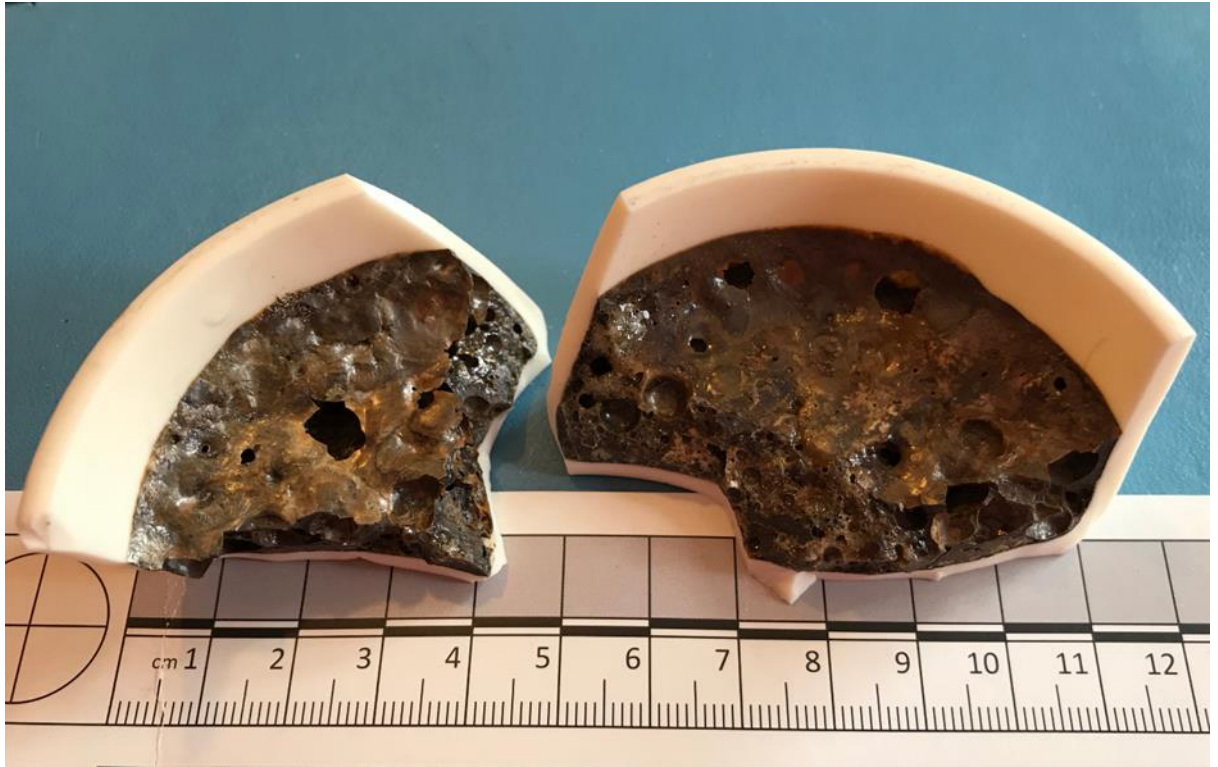
Figure 40: Pelitic melt at 1400°C.
