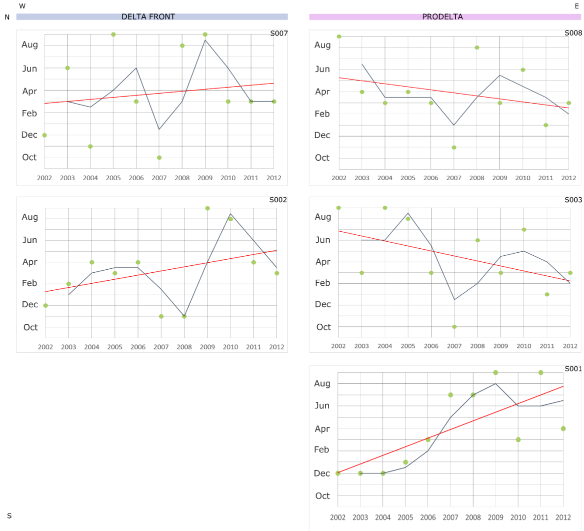
Figure 5.5. Evolution in time of maximum TSM concentration, linear and moving average trends for the studied period, in each of the five locations
