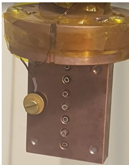
Figure 5.3. Photograph of completed OFHC copper cryostat mount prepared for introduction to the beam, ID18, ESRF, July 2018 (photograph credit: D. Wood).
