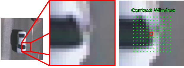
Figure 1: Context window used to evaluate each pixel in the Pixelwise network. All the pixels marked in green are used as the context of the pixel marked as red.
