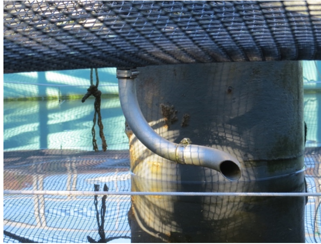
Figure 4-2 Rotating arm for distributing feed from the centre of tank
