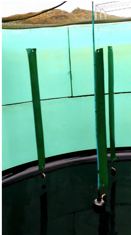
Figure 5-4 Artificial kelp suspended in tank and kept vertical by a weight at the bottom
