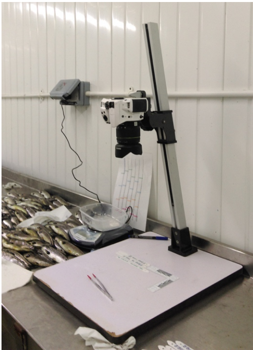
Figure 2-2 Photographs of the sampling set up showing camera affixed to an adjustable mount and an example of an image used to obtain physical measurements, see text for details.
