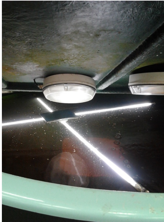
Figure 3-6 Fluorescent lights floating on the surface of the water, in the tank. Two further lights attached to tank lid (Photo courtesy of Sonia Rey)
