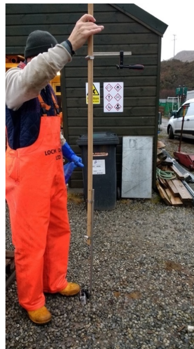
Figure-5-7 Camera in waterproof housing attached to the bottom mounting pole
