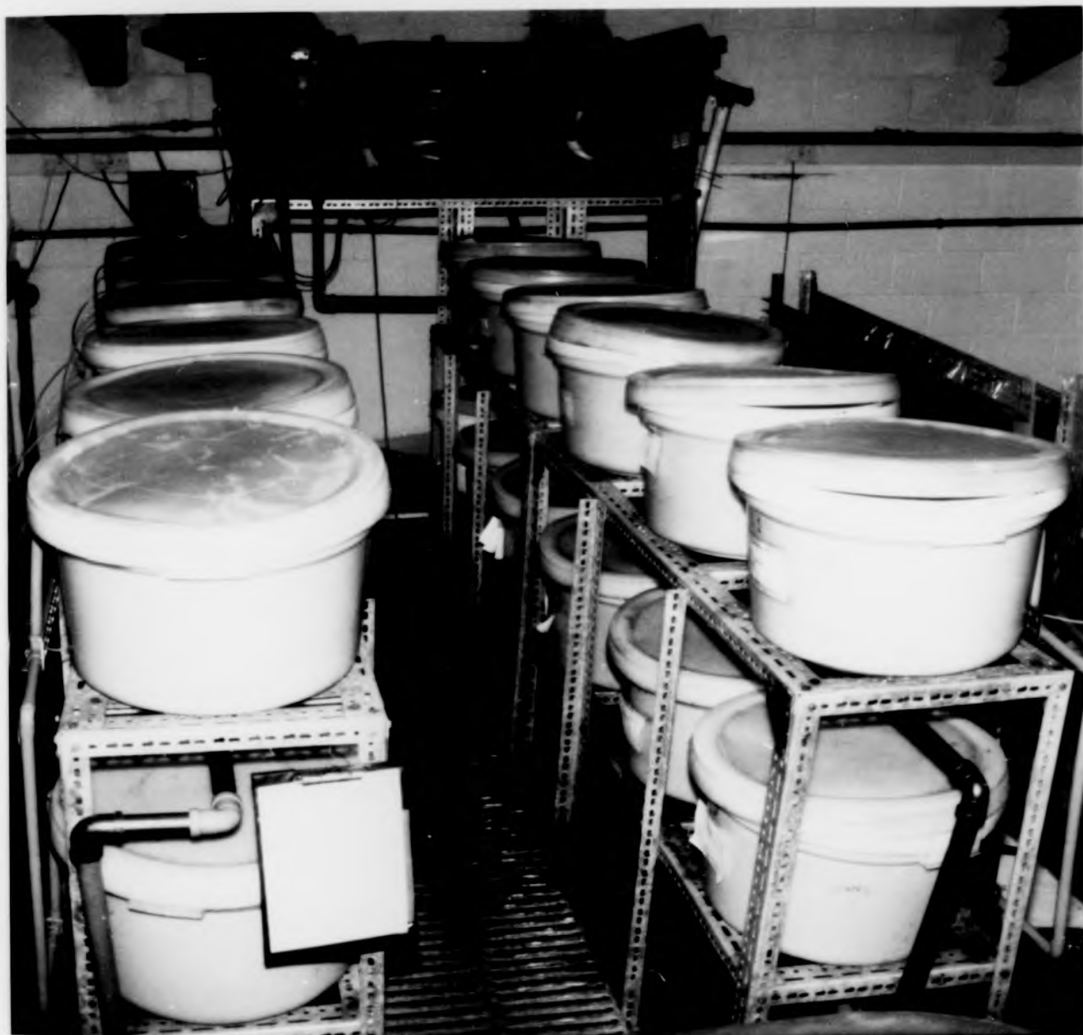
FIG. 1 Recirculated warm water system used for the growth studies
