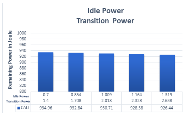
FIGURE 11. Levels of energy consumption of CALI in buffering mode against the value variations of idelPower and transitionPower energy parameters.
