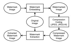
Fig. 1: Image security evaluation using watermarking.
