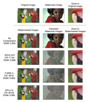
Fig. 3: Representative visual results of DCT watermarking with compression coding options (no compression, JPEG with quality 70, F-MSE-8 [18] and HiFic-mi [19]). Column 1 shows compression ratios (CR) and SSIM values of watermarked images. For similar visual quality at high CR (for both learning based coding), watermarking information is severely affected.
