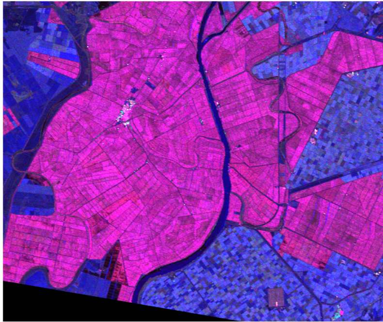
Figure 4.1: Rice fields in the South of Spain (Test site 1). Quad-Pol RADARSAT-2 image acquired the 02/08/2014. Blue: \sqrt{\lambda} \cos(\underline{\alpha}) , Red: \sqrt{\lambda} \cos(\underline{\alpha}) \sin(\underline{\beta}) , Green: \sqrt{\lambda} \sin(\underline{\alpha}) \sin(\underline{\beta}) (See equation 4.9).
