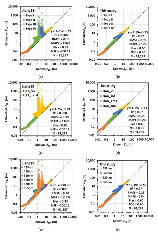
**Figure 4.** Comparison of known and estimated  $Z_{SD}$  values. The estimated  $Z_{SD}$  values were obtained from the simulated  $R_{rs}(\lambda)$  in Synthetic Dataset I using the Jiang19 algorithm (**a**,**c**,**e**) and the new algorithm proposed in this study (**b**,**d**,**f**). The colors in the figures represent water types (**a**,**b**), the QAA used (**c**,**d**), and the wavelengths with the minimum  $K_d(\lambda)$  (**e**,**f**).
