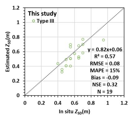
**Figure 6.** Comparisons of the in situ measured  $Z_{SD}$  values and the estimated  $Z_{SD}$  values from MERIS data using the new  $Z_{SD}$  estimation algorithm.
