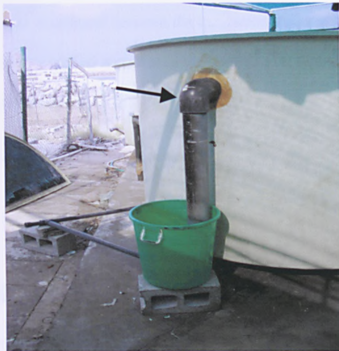
Figure 6.2 Egg collection mesh was placed at the outflow in the broodstock tank (arrow).
