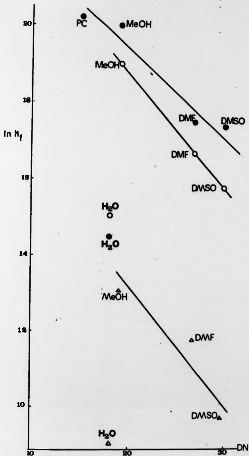
Figure 37 Formation Rate Constants for  $K(2,2,2)^+$  (●),  $Na(2,2,1)^+$  (○) and  $Li(2,1,1)^+$  (Δ) as a function of Solvent Donor Number
