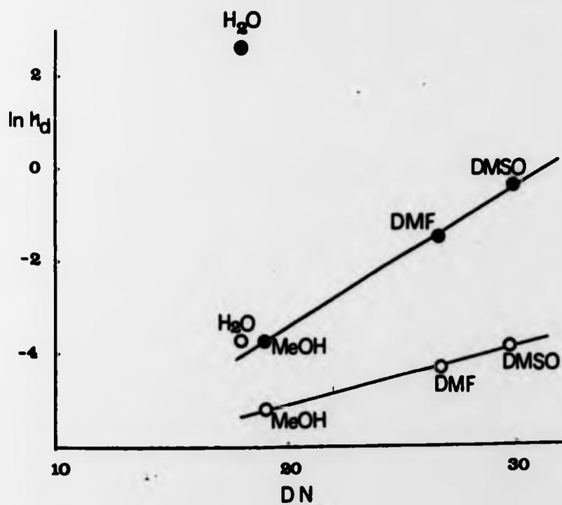
Figure 36 Dissociation Rate Constants for  $\text{Na}(2,2,1)^+$  (●) and  $\text{Li}(2,1,1)^+$  (○) as a function of Gutmann's Donor Number of the Solvent
