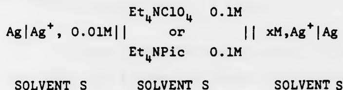
The potential readings were taken with a digital voltmeter (SOLARTRON A210).  $\text{Et}_4\text{NClO}_4$  (tetraethylammonium perchlorate) or  $\text{Et}_4\text{NPic}$  (tetraethylammonium picrate) was used in the salt bridge joining the two half cells. Both the detecting and the reference electrodes were  $\text{Ag}|\text{Ag}^+$  electrodes.
