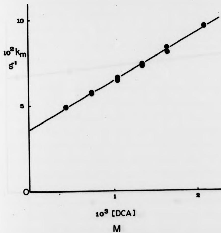
Figure 27 Dependence of  $k_m$  on [DCA] for the dissociation of  $K(2,2,1)^+$  in PC
