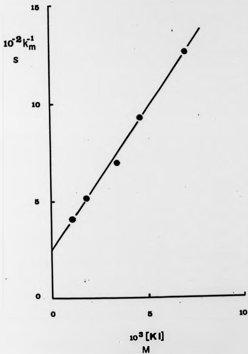
Figure 17 Dependence of  $k_m^{-1}$  on  $[KI]$  for the dissociation of  $K(2,2,2)^+$  in EtOH
