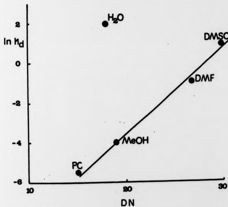
Figure 35 Dissociation Rate Constant for  $K(2,2,2)^+$  as a function of Gutmann's Donor Number of the Solvent
