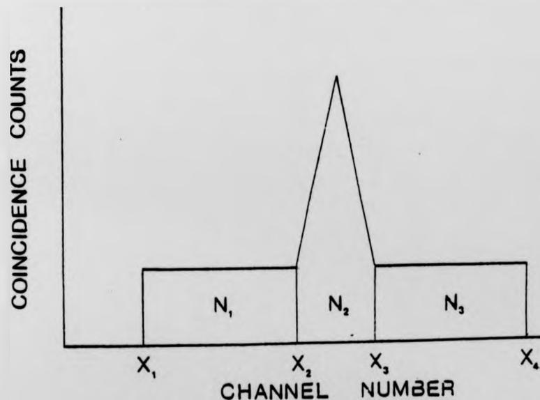
Fig. 4.15 Data acquisition for coincidence analysis
