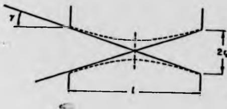
Fig. 3.5 Dashed lines show ideal space charge limited beam profile required to saturate a given space.
