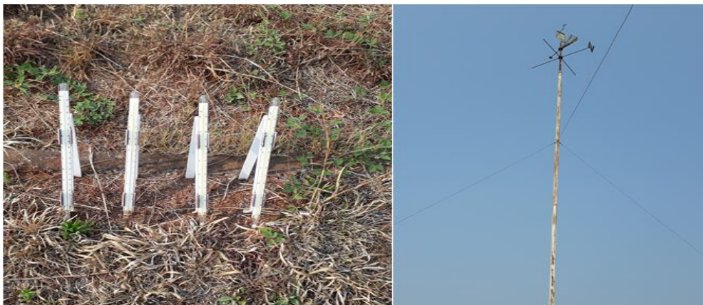
Figure 3.3 - Chianga terrestrial conventional weather station in Huambo province, Angola thermometers to measure air humidity and Wind direction indicator
