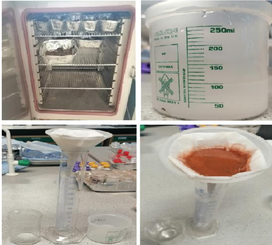
Figure 4.4. Soil water holding capacity determination using percolation method.
