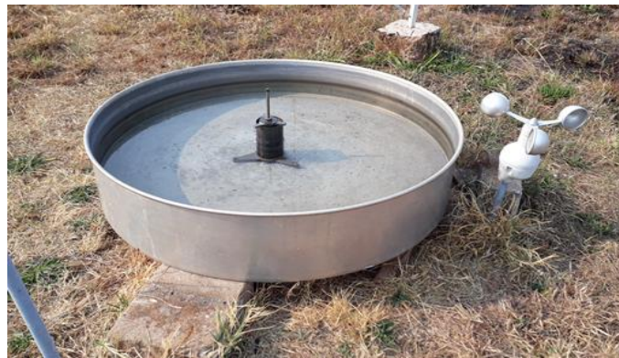
Figure 3.4 - Circular Pan for measuring evaporation in soil surface in Chianga weather station.
