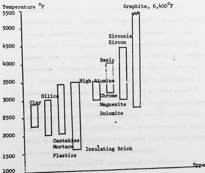
Figure F1: Service Temperature ranges of various refractories
