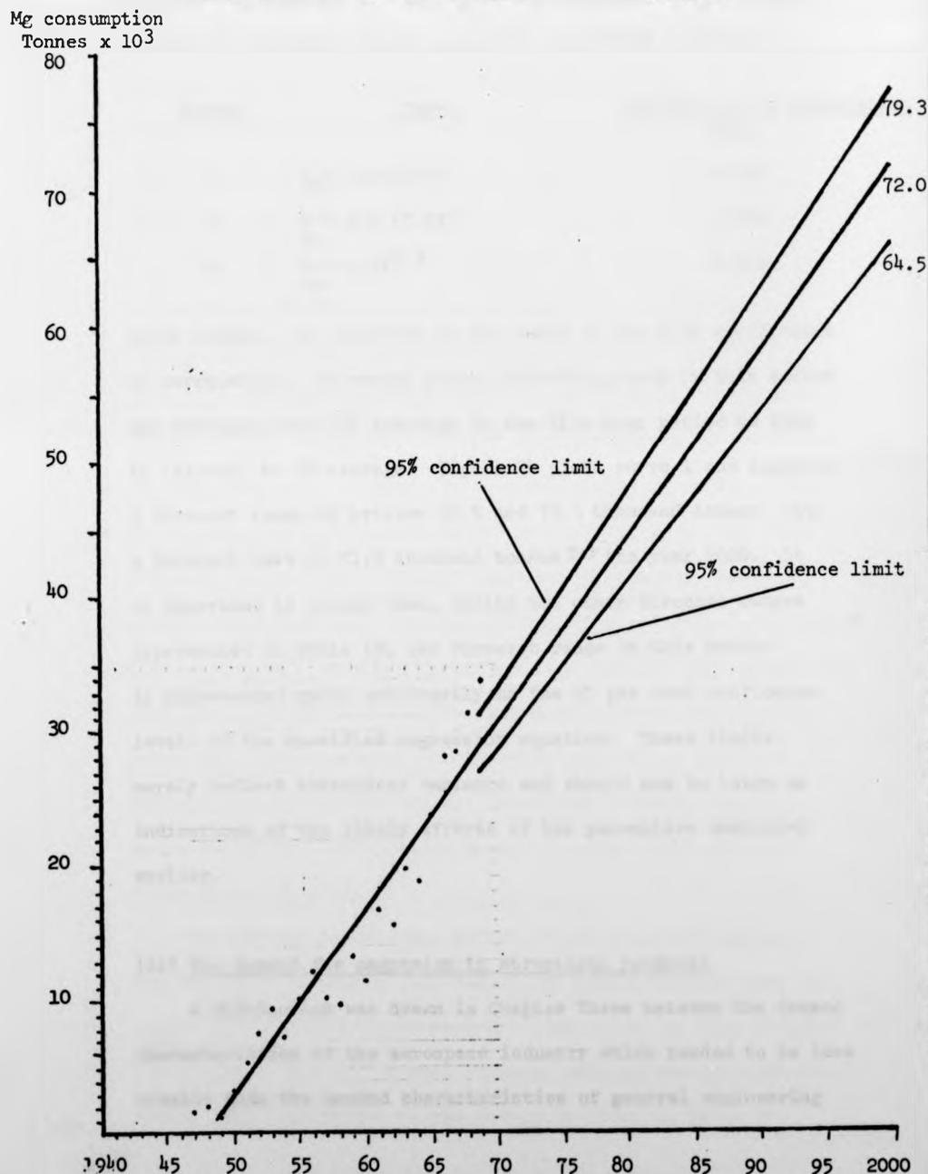
Equation:  $Y = 1.38X - 65.8$  where  $Y =$  consumption in tonnes x 10<sup>3</sup>,  $X =$  Year
