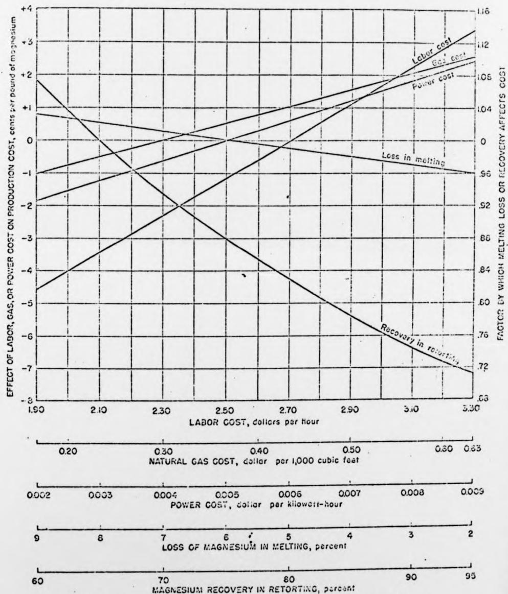
NOTE: Apply effect of labor, gas, or power cost (left ordinate) before applying factors for melting loss or recovery (right ordinate)
