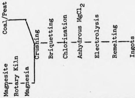
the relative economic importance of these preliminary stages of the production process is not crucial. Figure E1 provides some basic information on the structure of alternative production processes. All cost figures in this appendix:
