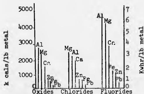
Minimum energy required to liberate lb of metal from various oxides and halides at 15°C
