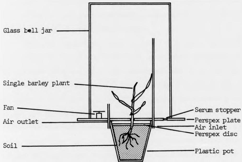
Fig. 40. Diagram of photosynthesis assimilation chamber.
