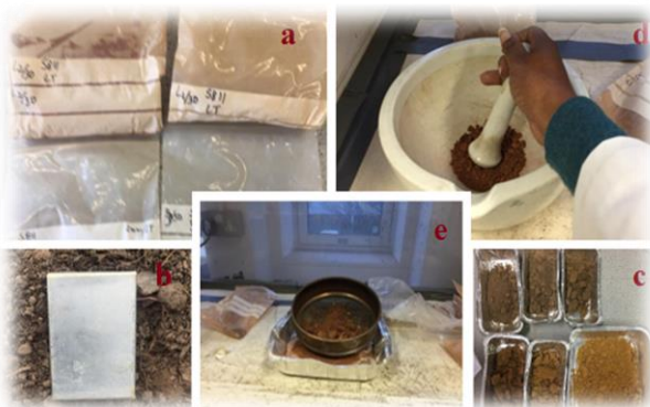
Figure 3. 13: a-deformed samples packed; b-undisturbed samples in Kubiena; c-samples ready for drying; d-sample grinding; e-sieve sample
