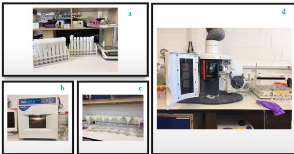
Figure 3. 16: Instrument laboratory (University of Stirling). A) vials; b) sample solution digestion; c) sample solution decanted; d) ICP equipment.
