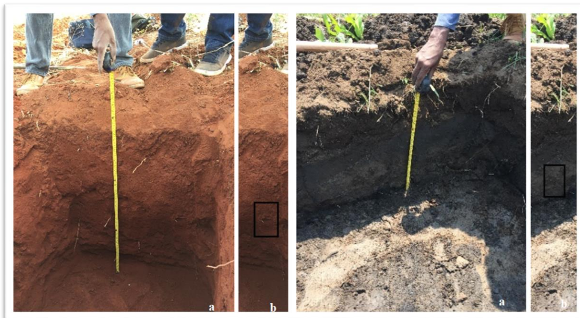
Figure 3. 7: a-open trench for sample collection (M2); b-undisturbed sample collection site for making slides (M2); c- open trench for sample collection (M3); d-undisturbed sample collection site for making slides (M3)-Mungo
