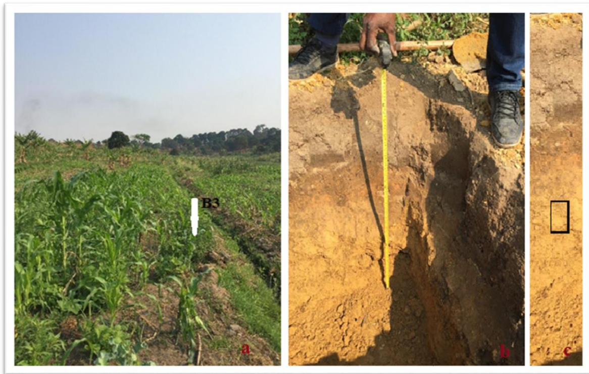
Figure 3. 6: a-B3 profile collection area; b-open trench for sample collection; c-undisturbed sample collection site for making slides-Bailundo
