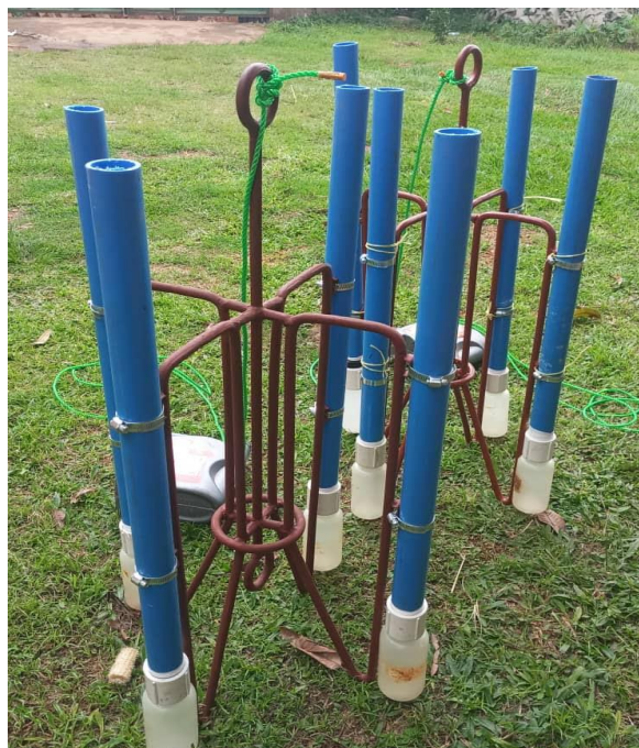
Figure 6.4: Sediment trap fabricated using locally available material. The painted iron bars were susceptible to rusting if available steel provides a better option.
