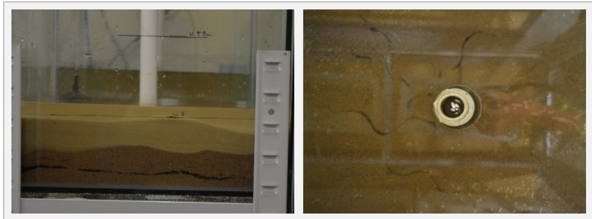
Figure 5.4 Tank set up and underside image showing burrowing experiments to monitor movement of lamprey larvae in experimental tank units.
