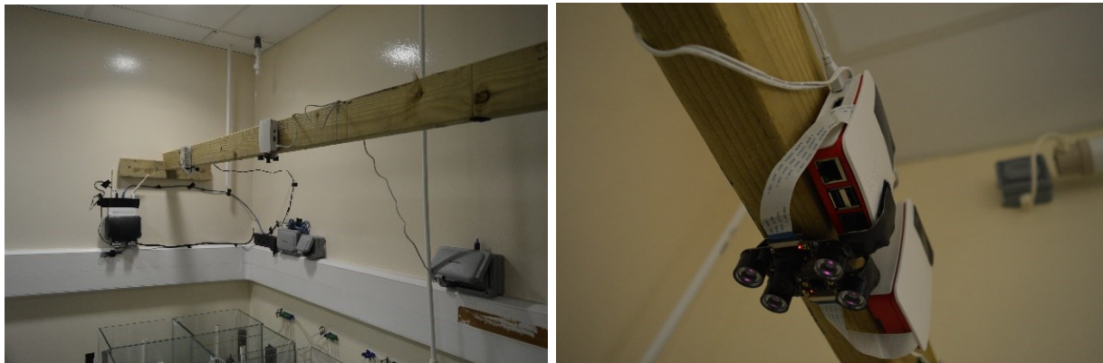
Figure 5.2 Set up of laboratory surveillance system with Raspberry Pi. RPi camera positioned above the tank to capture video images of the movement of larvae above the sediment, during both day and night.
