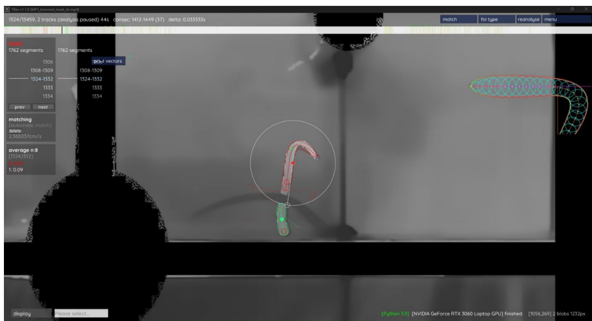
Figure 5.17 Trex open-source tracking software with a split lamprey in red and green in the centre. The substrate disturbance from the larva's previous position in the tank was being picked up by the software to identify multiple animals. The black shapes show the mask created in OpenCV is visible to reduce background noise.
