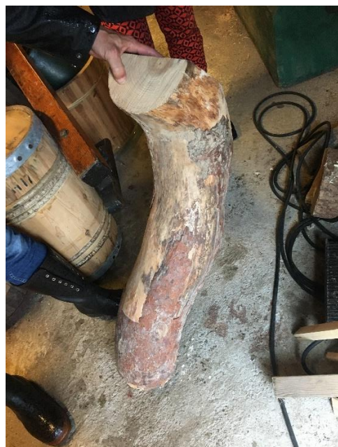
Figure 27. Curved branch for boatbuilding
