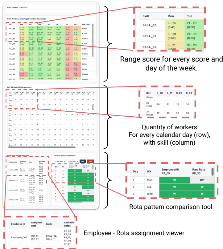
Figure 10.1: Best solution viewer tools, available to our industrial collaborator during the interview. The fitness function is broken into its summands (range scores for every combination of skill and weekday), and these are shown as a heatmap (top of figure). These range scores are based on how many workers with each skill appear throughout the 3 month period, as shown in the mid-section of the figure. The rota assignments for each worker, along with other rota patterns available and skillset, are shown in the bottom-left of the figure. The user was able to compare rota patterns (bottom-right).
