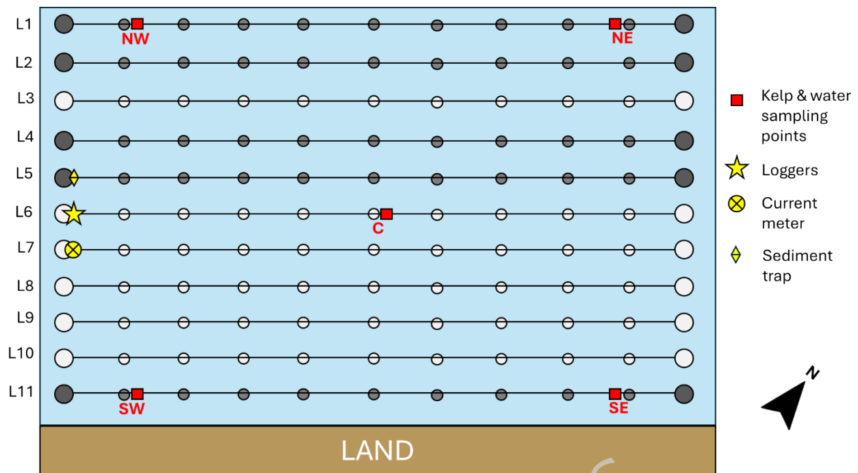
Fig. 8 Detailed sampling layout of kelp farm. Grey circles indicate buoys making up kelp lines (large: mooring buoy; dark grey: intact line; light grey: line damaged by storms in 2024). Red blocks indicate kelp sampling points. Yellow star indicates location of PAR and temperature loggers. Yellow circle indicates location of current meter. Yellow diamond indicates location of sediment trap. Salmon farm located 200m to the west.
